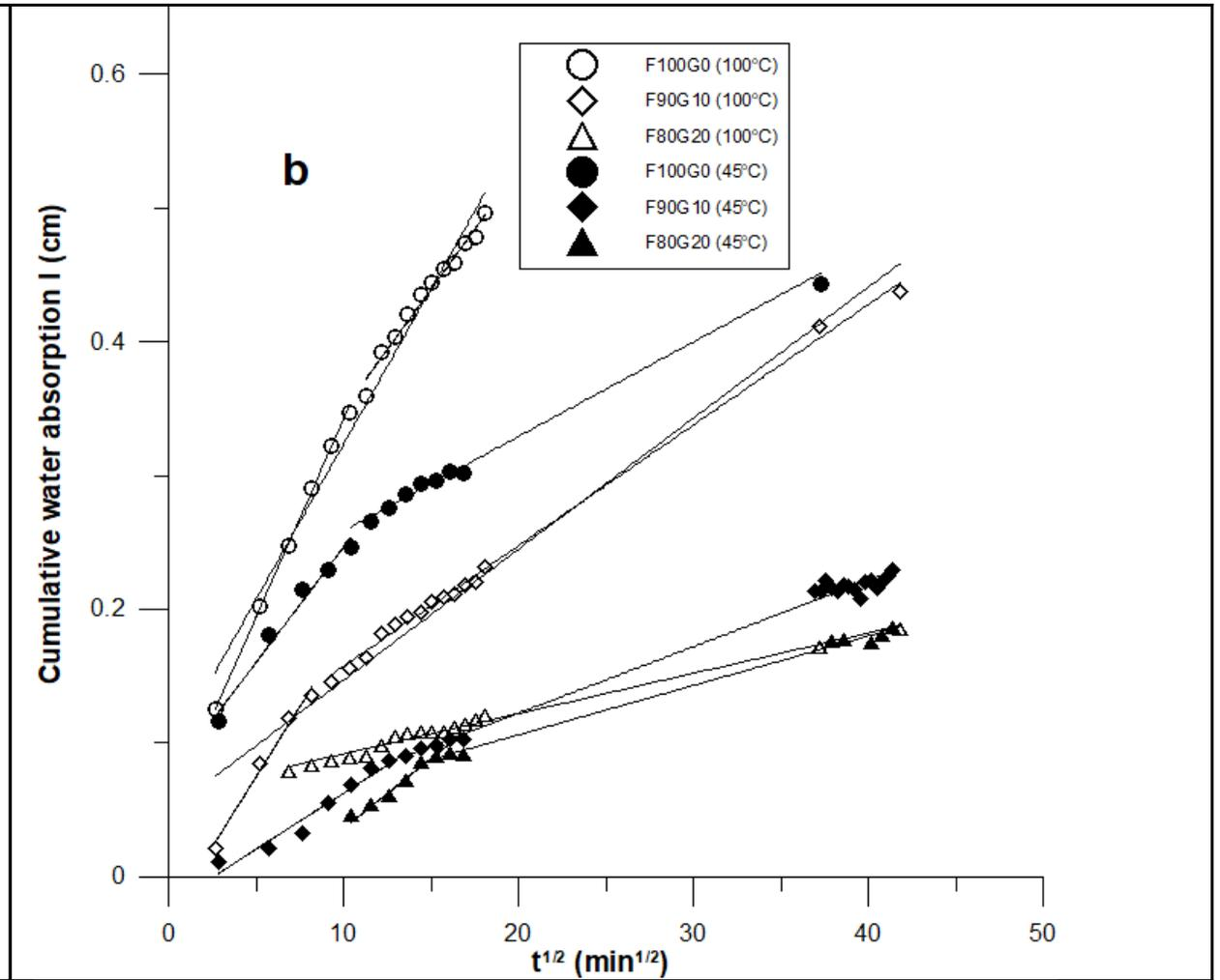
Progress of waterfront positions a) and cumulative water absorption I (b) versus the square root of absorption for fly ash- based mortar containing 0, 10, and 20% slag dried at 45<sup>0</sup> C and 100<sup>0</sup> C along with fit lines of straight-line equation
