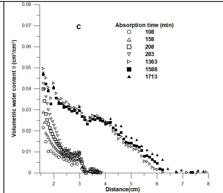
Water profiles for the mortar samples dried at  $45^{\circ}\text{C}$ : a) F100G0, b) F90G10 and c) F80G20.
