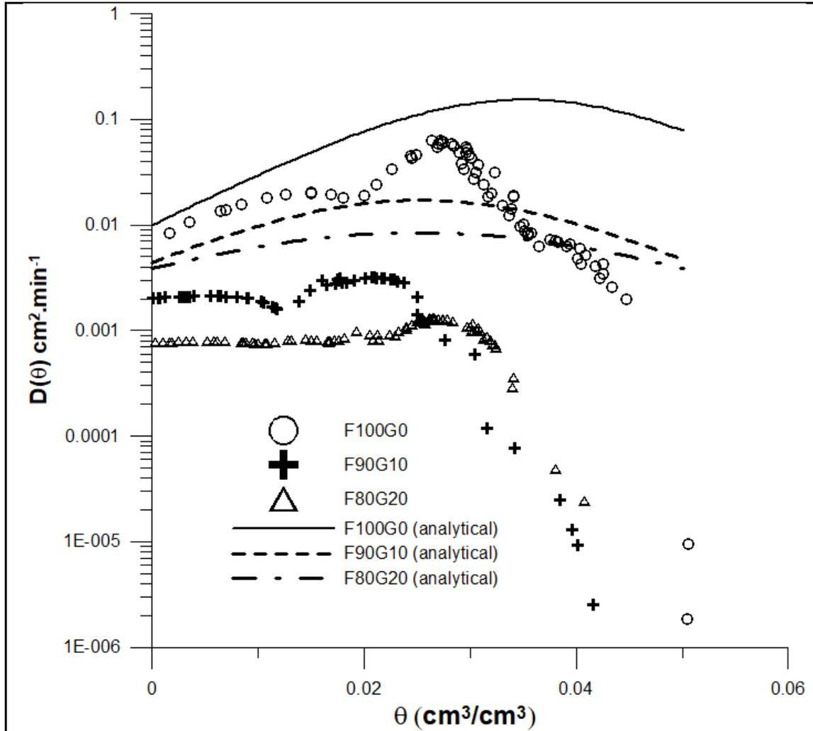
water diffusivity for the mortar samples dried at 45°C
