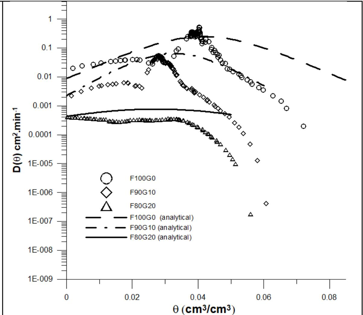
water diffusivity for the mortar samples dried at 100°C
