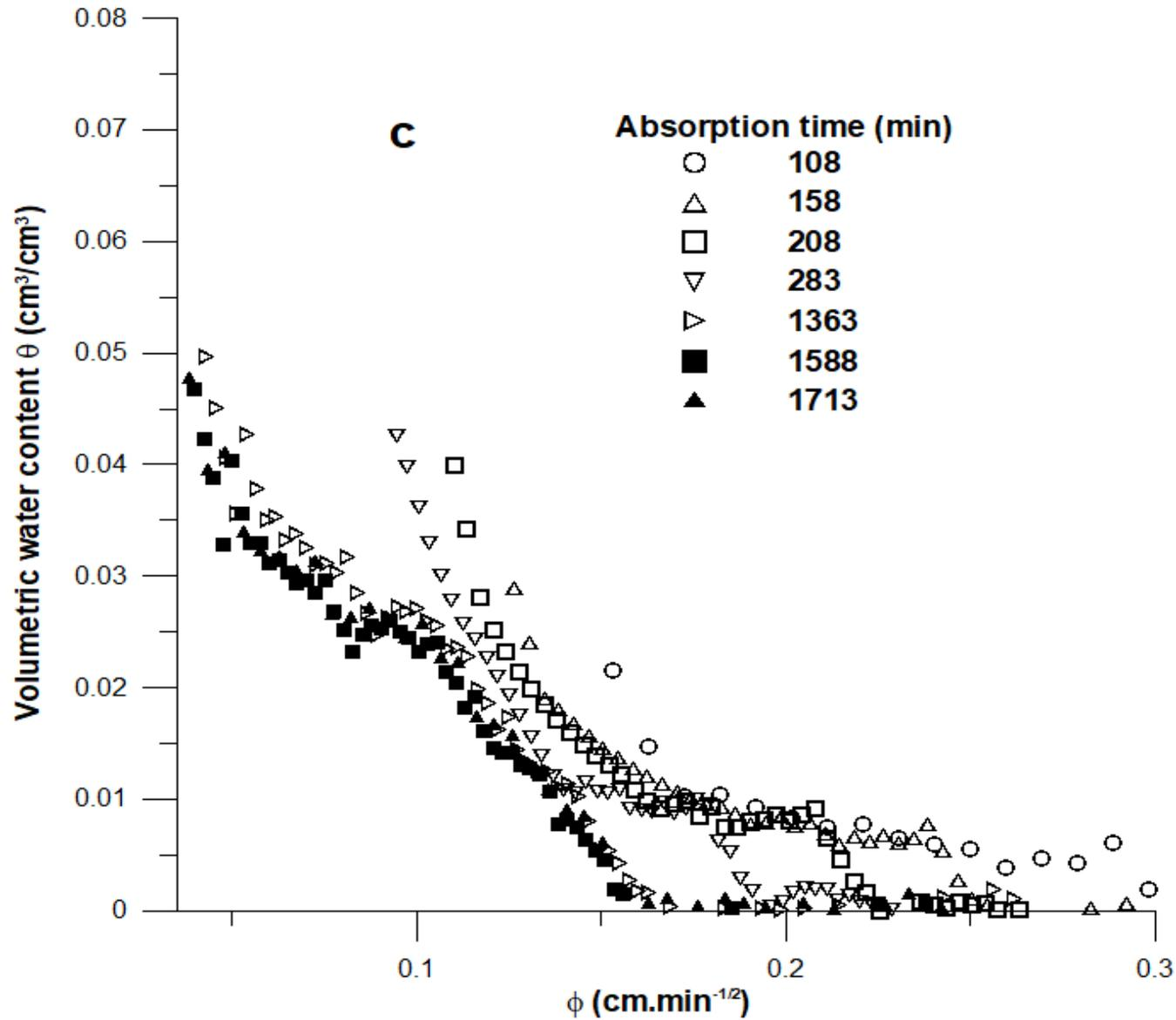
The  $\theta - \phi$  profiles for the F100G0, F90G10 and F80G20 samples dried at 45°C
