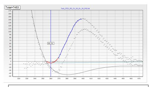
real 2-hit event, restoring original waveform from pile-up
