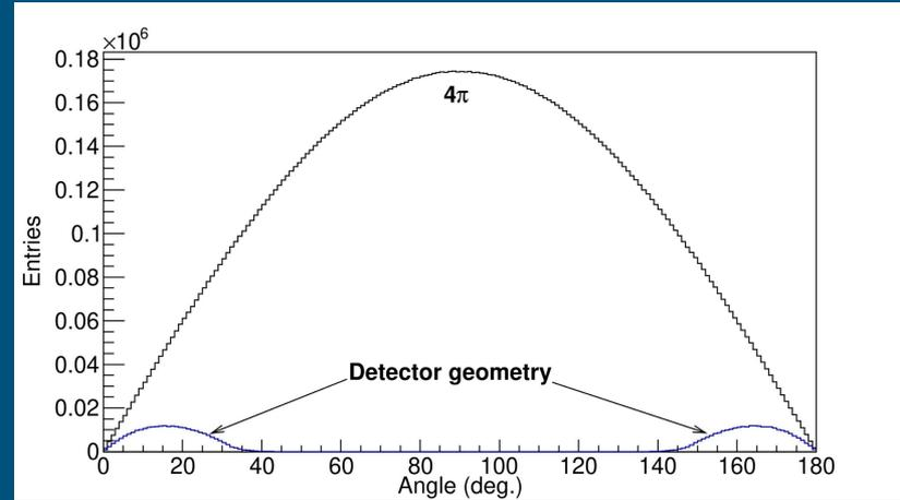
Simulation of the angle between two particles which can be detected in our detection system consisting of two telescopes
