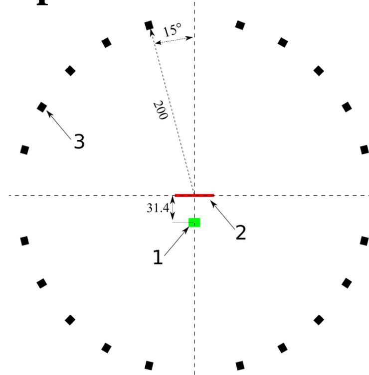
Fig. 4. Scheme of the TANGRA setup with plastic detectors for measuring angular distributions of the scattered neutrons. Designations as in Fig. 3. Dimensions are in cm.
