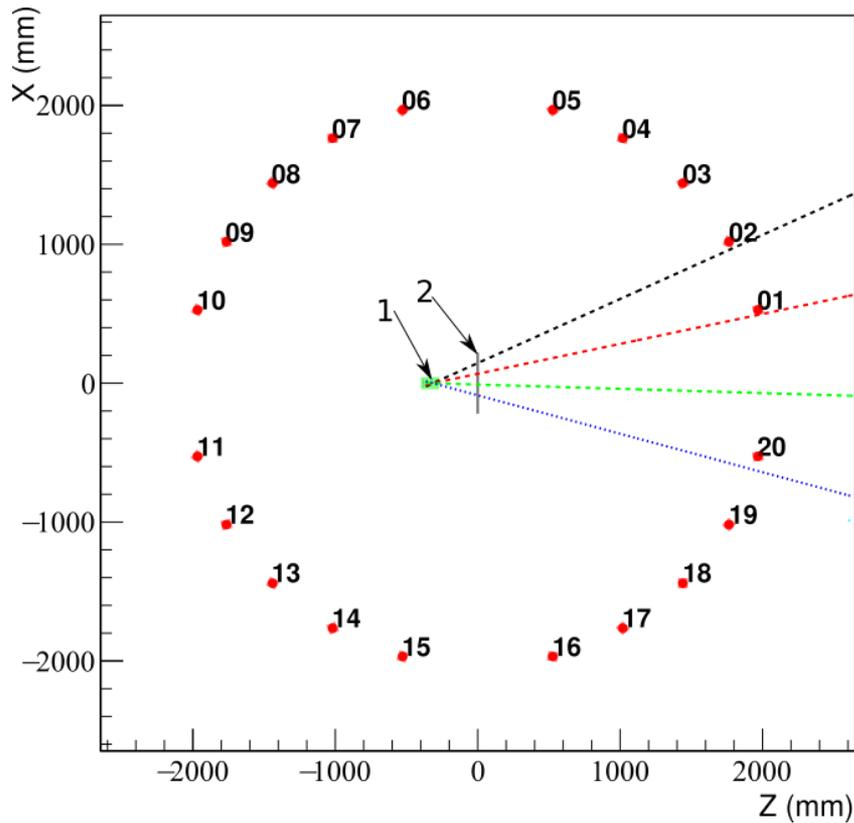
Fig. 8. Scheme of the TANGRA setup with some of “tagged” neutron beam’s. Where: 1 – is ING-27, 2 – target.
