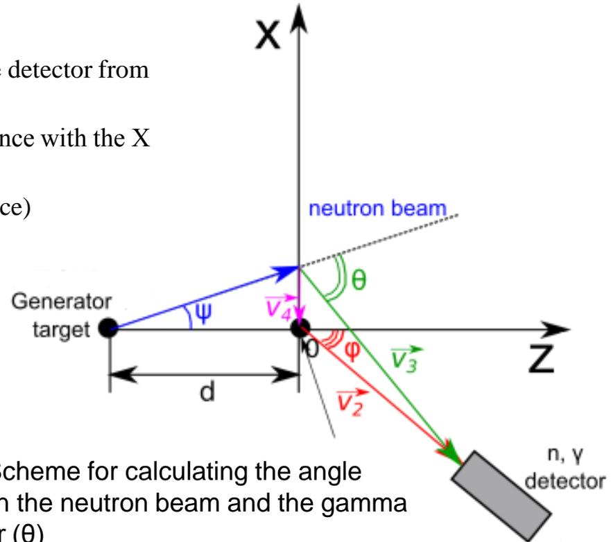
Fig. 9. Scheme for calculating the angle between the neutron beam and the gamma detector ( $\theta$ )
