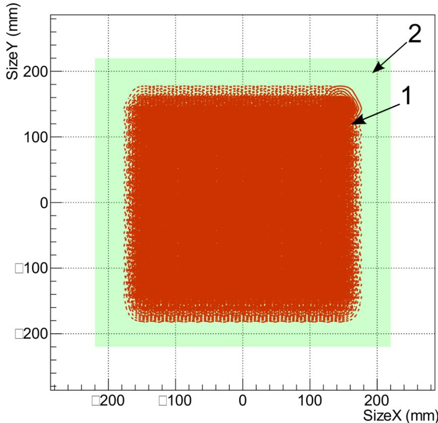
Fig. 8. Neutron beam 2D profile (1) on the target (2).
