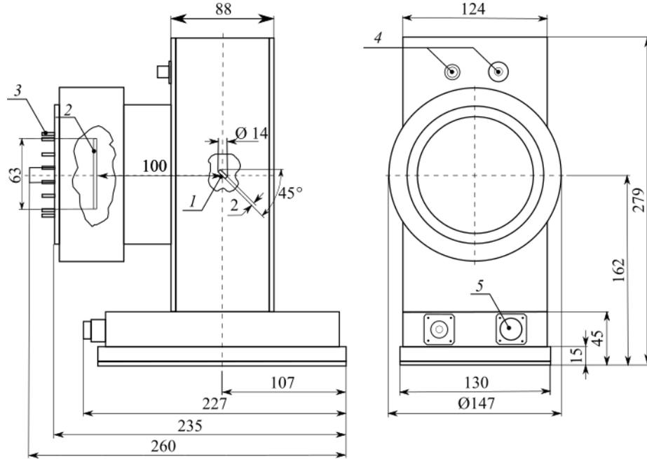
Fig. 5. 1 – neutron generator target, 2 –  $\alpha$ -detector, 3 – signal connector of  $\alpha$ -detector, 4 – high-voltage power connectors, 5 - low-voltage control connector
