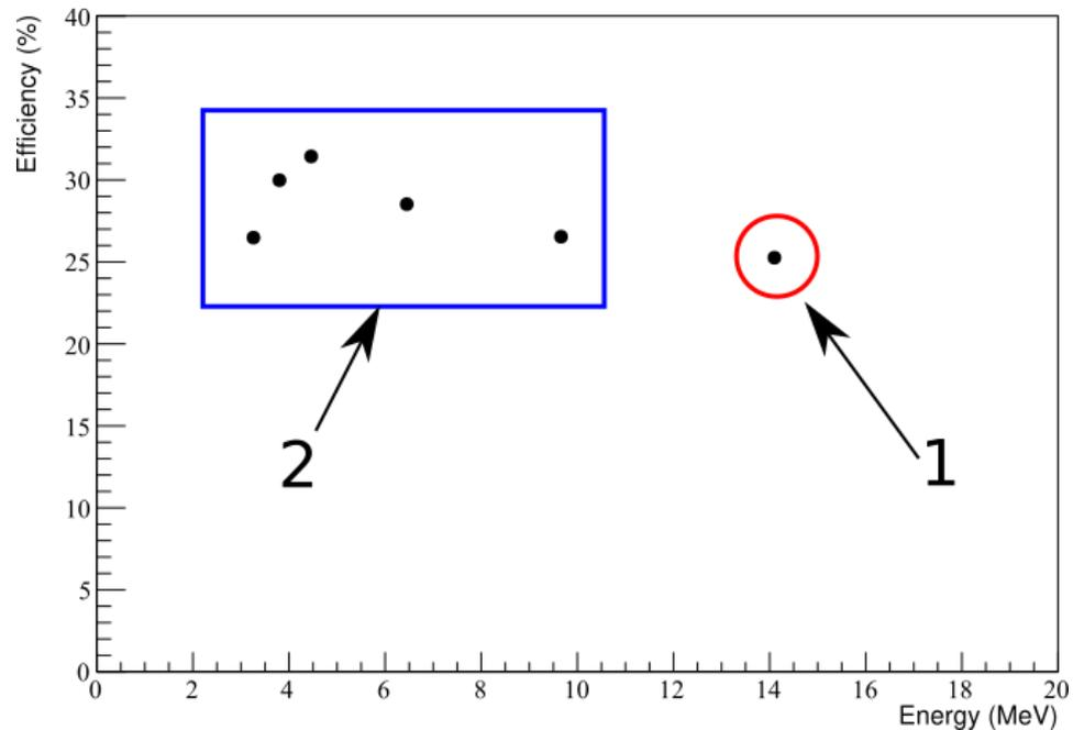
Fig. 11. Geant4 intrinsic efficiency  $\epsilon$  (%) for neutrons with different energy. Where: 1 – is experimental measurement and 2 – modeling.
