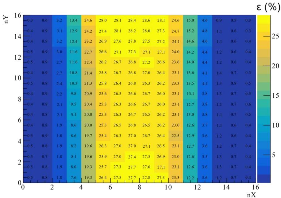
Fig. 10. Experimental intrinsic efficiency  $\epsilon$  (%) for 14.1 (MeV) neutrons for one detector
