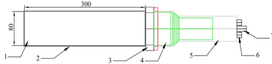
Fig. 6. 1 - plastic scintillator, 2 - reflective winding, 3 - aluminium holder, 4 - ETL9821KFLB photomultiplier, 5 - magnetic screen, 6 - BNC connectors (x2) and 7 - SHV connector.
