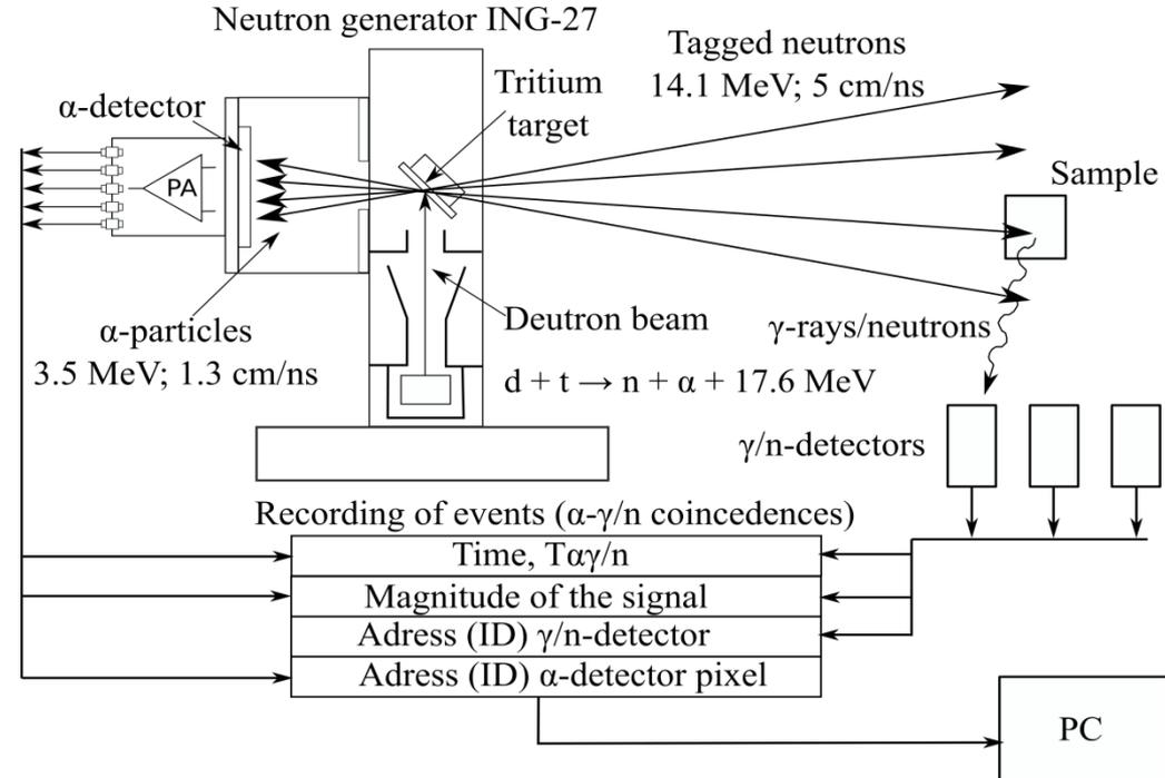
Fig. 1. Standard diagram of TANGRA experimental setups.
