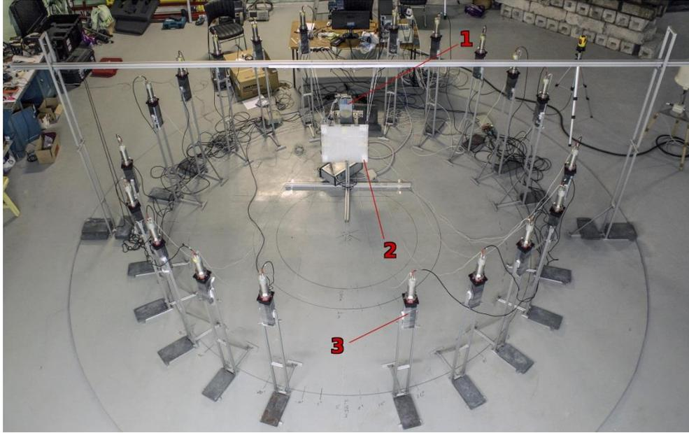
Fig. 3. Photo of the TANGRA setup with plastic detectors for measuring angular distributions of the scattered neutrons. 1 – ING-27 neutron generator, 2 – irradiated carbon sample, 3 – one of the 20 plastic detectors used in the registration system.
