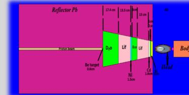
Figure (1): Final BSA model geometry configuration design and a human head model.
