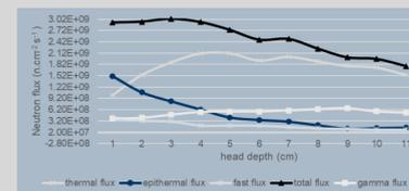
Figure (2): Neutron flux and gamma flux distributions along the head depth before <sup>10</sup>B injection.
