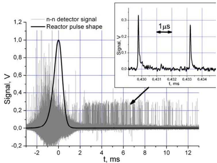
**FIGURE 6.** A signal from neutron detector (thin grey lines) in dependence on TOF. Each peak corresponds to neutron registration event. A black curve shows a time dependence of the reactor power during the pulse
