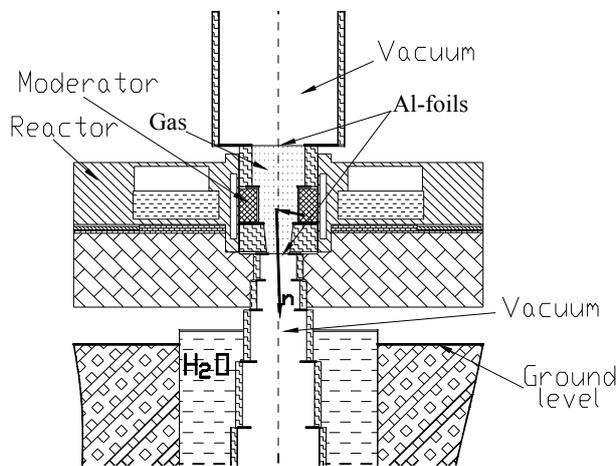
**FIGURE 7.** The scheme of measurements with noble gases
