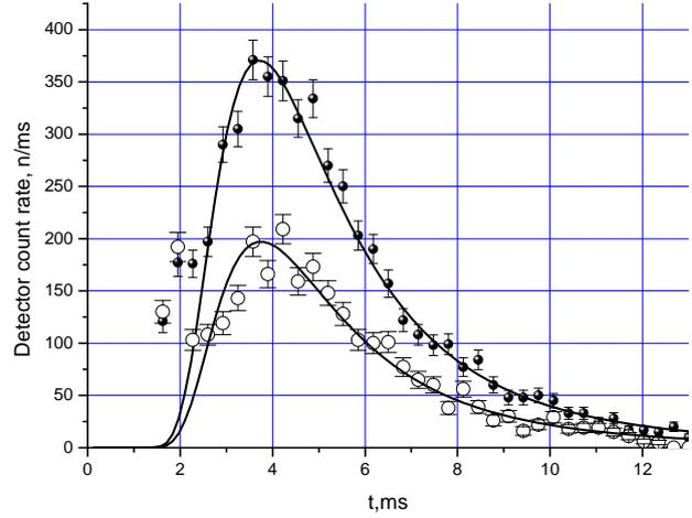
**FIGURE 10.** The TOF spectra measured with vacuumed scattering chamber for 31 MJ (black points) and 25MJ (open circles). The curves are a fit with Maxwellian distribution.
