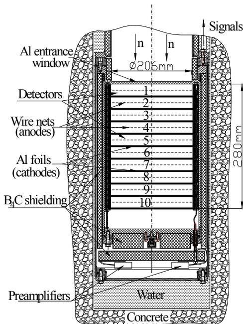
**FIGURE 5.** The layout of the neutron detector
