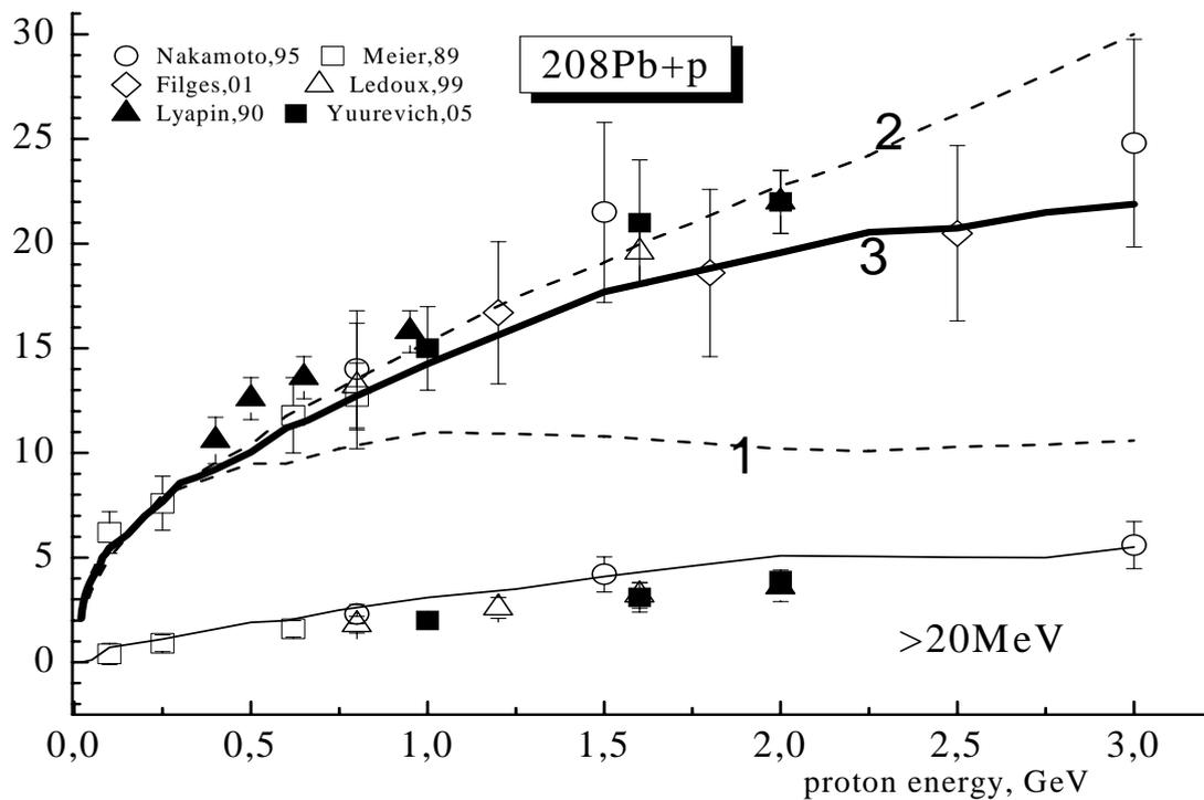
Fig. 6. The neutron multiplicities of  $208\text{Pb} + p$  reaction. The symbols are the experimental data. The dashed lines are the results of calculations with the fixed  $M_n = 5$ ,  $M_p = 2$  (curve#1) and with  $M_n = 25$ ,  $M_p = 10$  (curve # 2). The results of calculations with fixed maximal preequilibrium configuration are shown by solid curve # 3.
