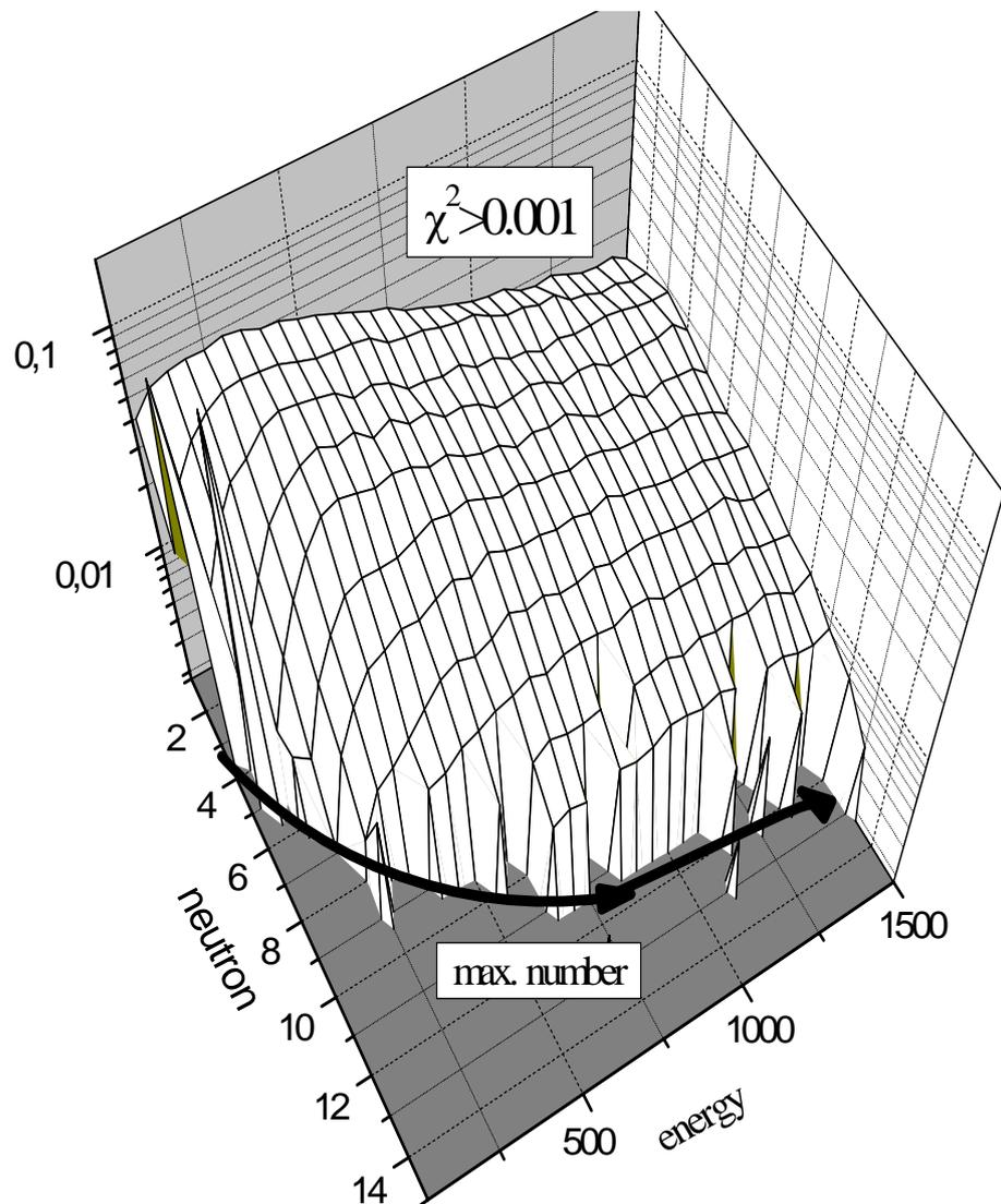
Fig. 5. Deviations of the neutron spectrum shape from equilibrium one depending on neutron serial numbers and on proton energy. The line shows the maximal number of nonequilibrium neutrons.
