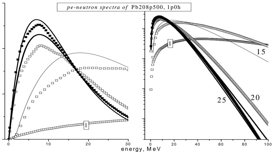
Fig. 3. Calculated spectra of neutrons from various particle-hole configuration (symbols) and the spectra calculated with evaporation model (lines). Numbers designate states.
