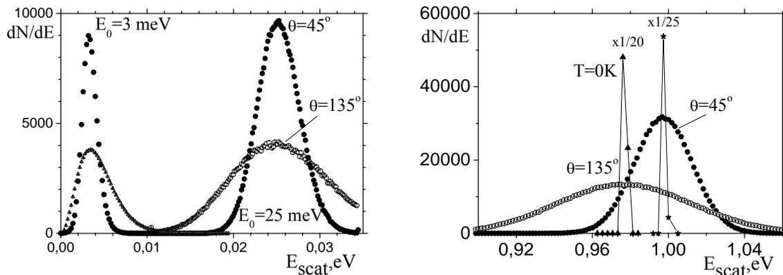
Fig.3. Distribution of neutrons with initial energies 0.003 eV, 0.025 eV and 1 eV scattered by krypton. In the right picture the distributions of neutrons scattered by immovable gas ( $T=0^{\circ}\text{K}$ ) are shown also (narrow peaks).
