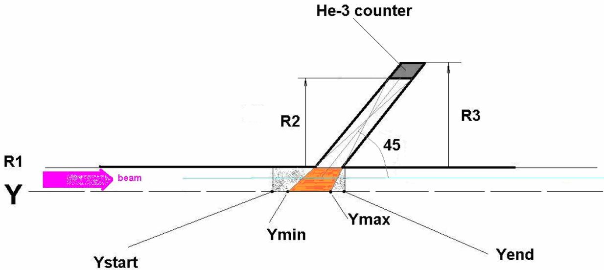
Fig.2. The scheme for Monte Carlo calculations for neutrons scattered forward. The calculating parameters: radius of the falling neutron beam  $R1=2$  cm, inner radius of detector ring  $R2=21.213$  cm, outer radius of detector  $R3=24.213$  cm.
