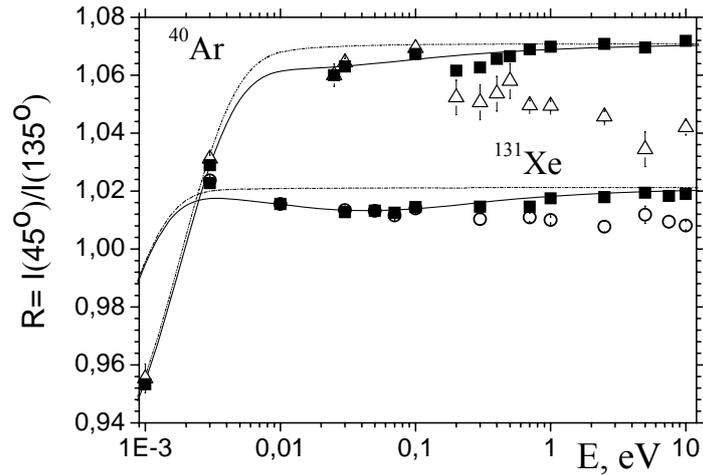
Fig.5. The scattering anisotropy dependence on neutron energy for argon and xenon: open circles and triangles are calculations without correction for efficiency, squares are the calculations with this correction. Solid curves are analytical calculations with taking into account  $b_{ne}$  value, dashed curves are ones with  $b_{ne}=0$ .
