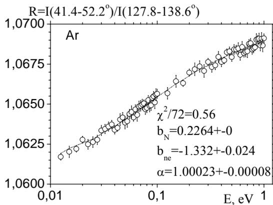
Fig.6. The result of fits for argon. Open points are pseudo-experimental data, dashed curve is the fitting curve.
