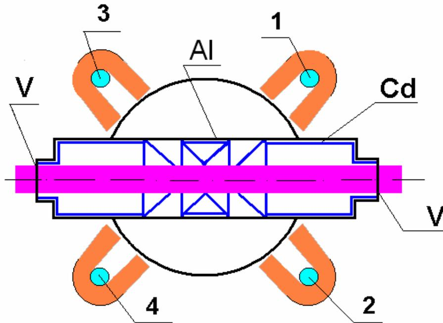
Fig.1. The installation scheme: 1,2,3,4 –  $^3\text{He}$ - counters in borated polyethylene shielding fixed to the round turn-table.
