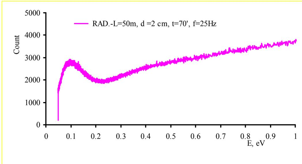
**Fig. 6.** Energy dependence in the TOF spectrum of the open beam, measured on the 50 m flight path of the central channel of the RADEX setup (time channel width 4  $\mu$ s in 4096 channels  $t = 16384 \mu$ s)
