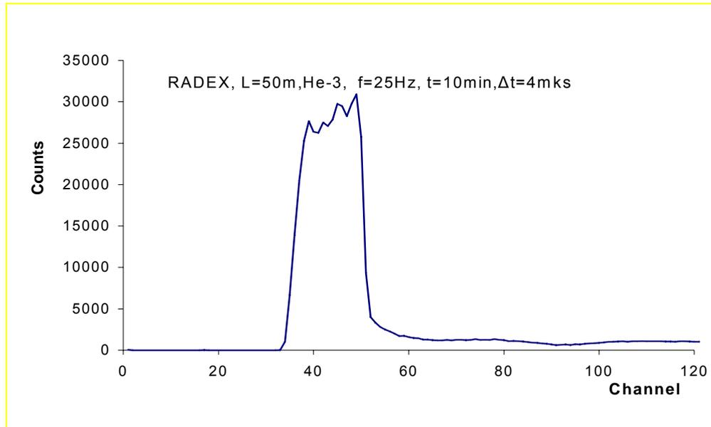
**Fig. 8.** TOF spectra of the open beam, measured on the 50 meter flight path of the central channel of the RADEX setup (time channel width  $4 \mu\text{s}$  in 4096 channels  $t = 16384 \mu\text{s}$ )
