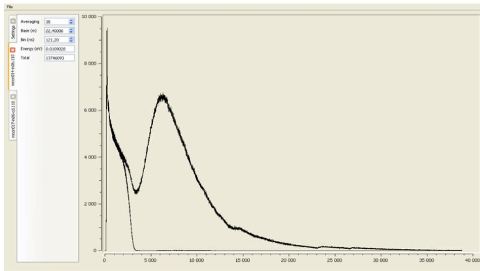
**Fig 5.** TOF spectra of the open beam and TOF spectra with cadmium sample, measured on the 22.4 m flight path of the first channel of the IN-06 source (time channel width 21 ns in 321240 channels,  $t = 39500 \mu\text{s}$ )
