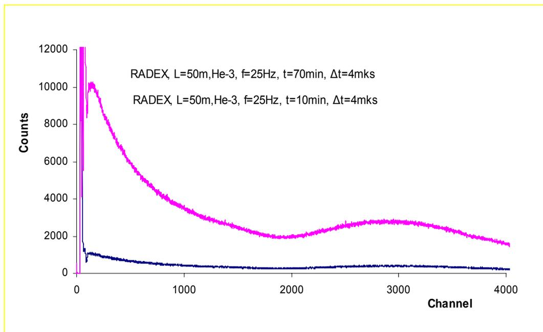
**Fig. 7.** TOF spectra of the open beam, measured on the 50 meter flight path of the central channel of the RADEX setup (time channel width 4  $\mu$ s in 4096 channels  $t = 16384 \mu$ s)
