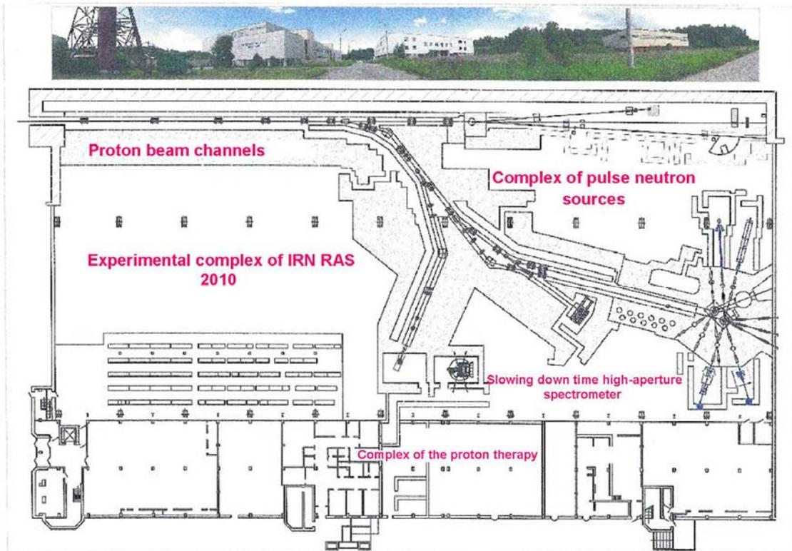
**Fig. 1.** A general scheme of pulsed neutron sources RADEX and IN-06 placement in experimental complex (building 25) of Institute of Nuclear Researches of the Russian Academy of Sciences.
