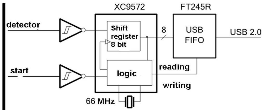
**Fig. 2** Functional scheme of the DAQ device
