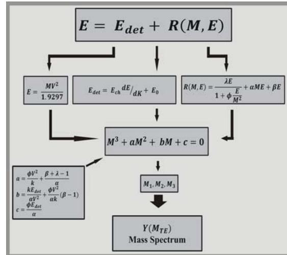
**FIGURE 7.** Processing of velocity- energy data for calculation of fragment mass. Code is based on parameterization [6] of pulse height defect in PIN diodes.
