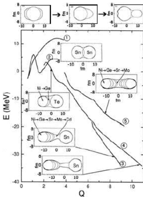
**FIGURE 4.** The bottoms of the fission valleys as a function of parameter  $Q$  (proportional to the quadrupole moment) for  $^{252}\text{Cf}$  nucleus. The panels depict the shapes of the fissioning system at the points marked by arrows. Valley 1 in the figure is due to preformation of double magic  $^{208}\text{Pb}$ . Evolution of the nuclear shape in this mode is presented above the figure.
