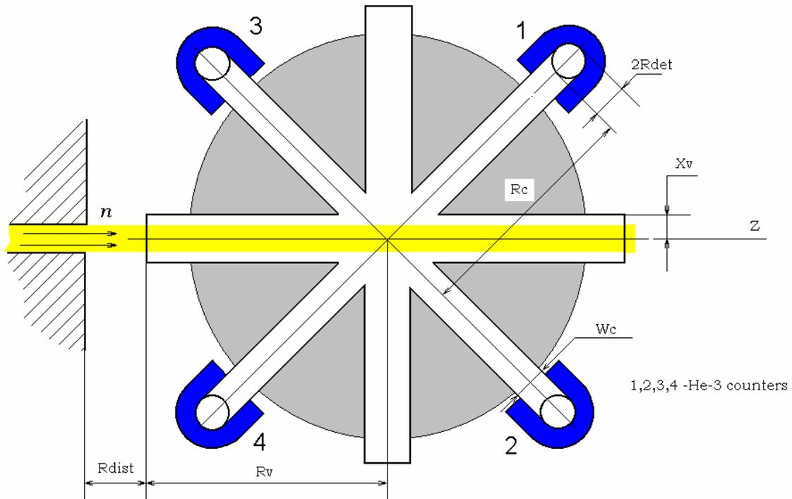
Fig.1. Scheme of the installation for calculating the neutron scattering (view from above).
