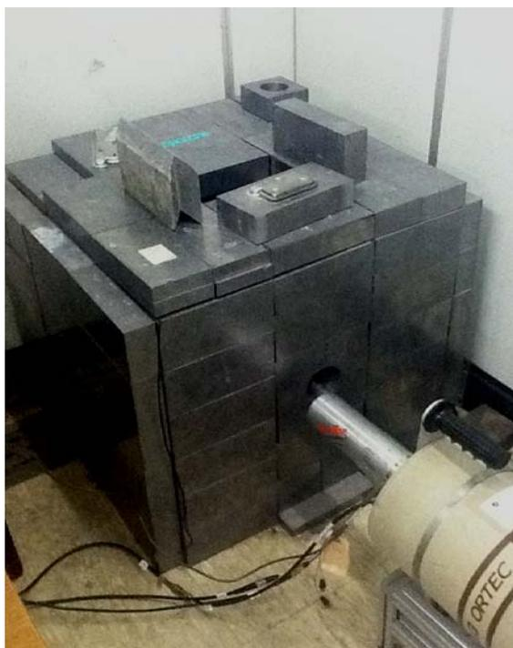
Fig.1. Detector and shielding box view
