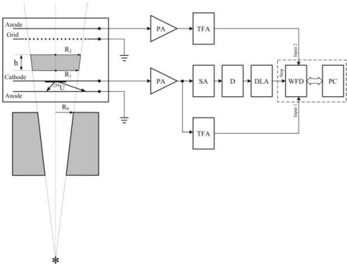
**Figure 1.** Scheme of experimental setup. PA – preamplifier, TFA – timing filter amplifier, D – discriminator, DLA – delay line amplifier, SA – spectrometric amplifier, WFD – waveform digitizer.
