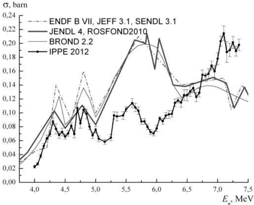
**Fig. 5.**  $^{19}\text{F}(n,\alpha)^{16}\text{N}$  reaction cross section in comparison with estimated data. Curve with closed circles – present work data, wide curve – JENDL 4, ROSFOND2010, fine curve – BROND 2.2, dash dot curve – ENDF B VII, JEFF 3.1, SENDL 3.1.
