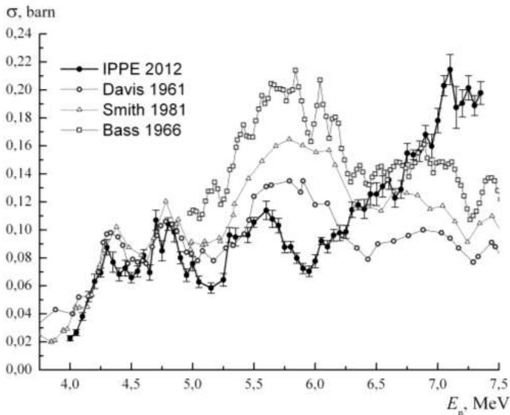
**Fig. 4.**  $^{19}\text{F}(n,\alpha)^{16}\text{N}$  reaction cross section in comparison with experimental data. Closed circles – present work data, opened circles – data of Davis 1961, opened triangles – data of Smith 1981, opened squares – data of Bass 1966.
