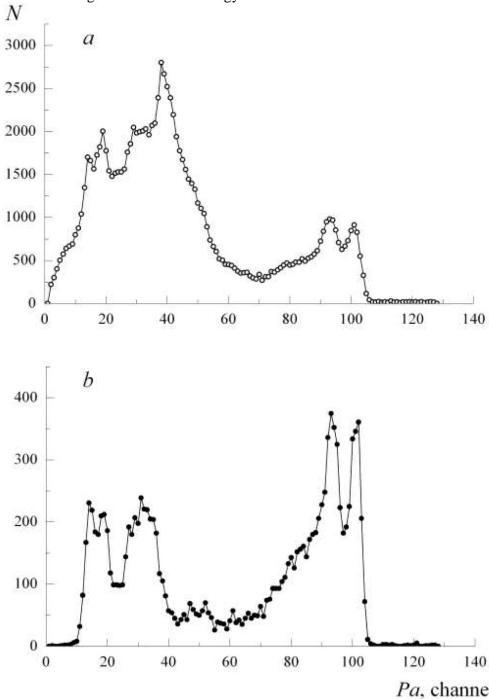
**Fig. 2.** *a* – anode signals spectrum of ionization chamber; *b* – the same spectrum after event selection.
