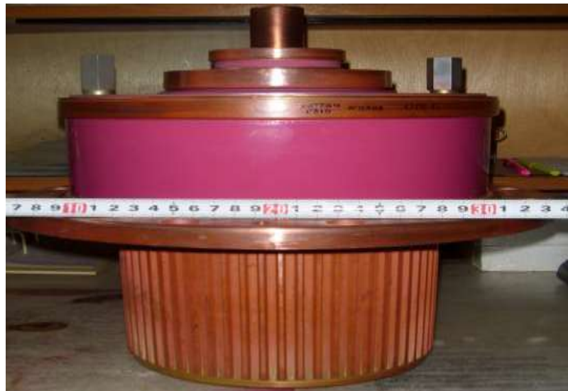
Fig.7. New metal-ceramic coaxial triode GI-71A of the exit RF amplifier cascade. ( f=198.2 \text{ MHz} , P=3 \text{ MW} ).
