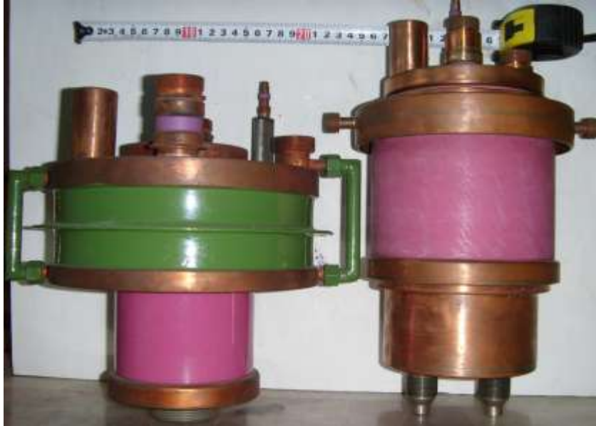
Fig.6. Electric vacuum lamps of preliminary amplifier cascade at the initial part of the accelerator. On the left side the old triode GI-51A is shown, on the right side new triode GI-57A is placed. ( P= 300 \text{ kW} , f=198.2 \text{ MHz} ).
