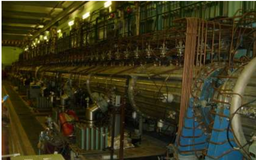
Fig.5. Initial part of the accelerator ( f = 198.2 MHz). A total length of the Alvarez resonators is 70 m.
