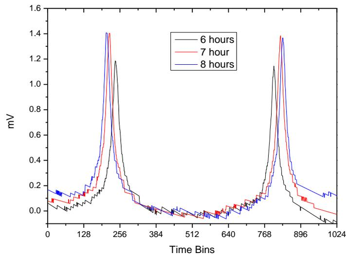
Figure 4. Typical NMR signal from polarized  $^3\text{He}$  as a function of pumping time.
