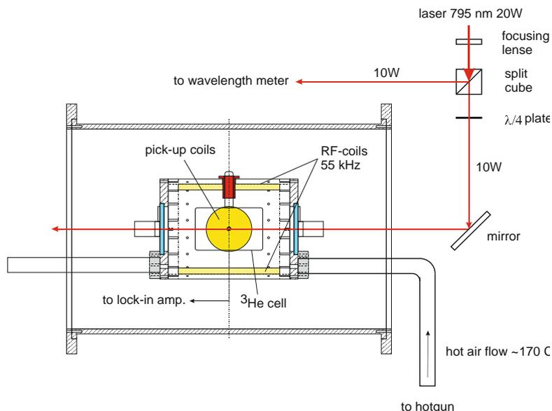
Figure 1. The sketch of  $^3\text{He}$  optical pumping facility.
