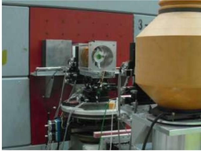
Figure 4. Polarized  $^3\text{He}$  cell on HANARO beam line for cold neutrons.
