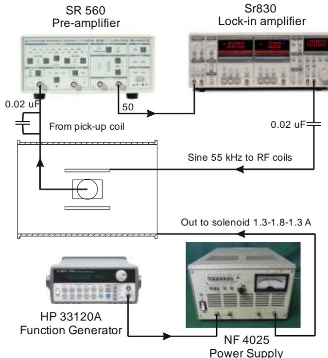
Figure 3. NMR signal measurement circuit.
