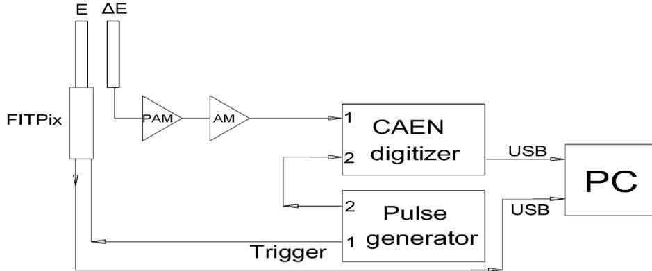
Fig.3. Experimental layout for time coincidence setup. The first channel of a dual pulse generator was used as external start for the FITPix interface. The second channel was used for synchronization.
