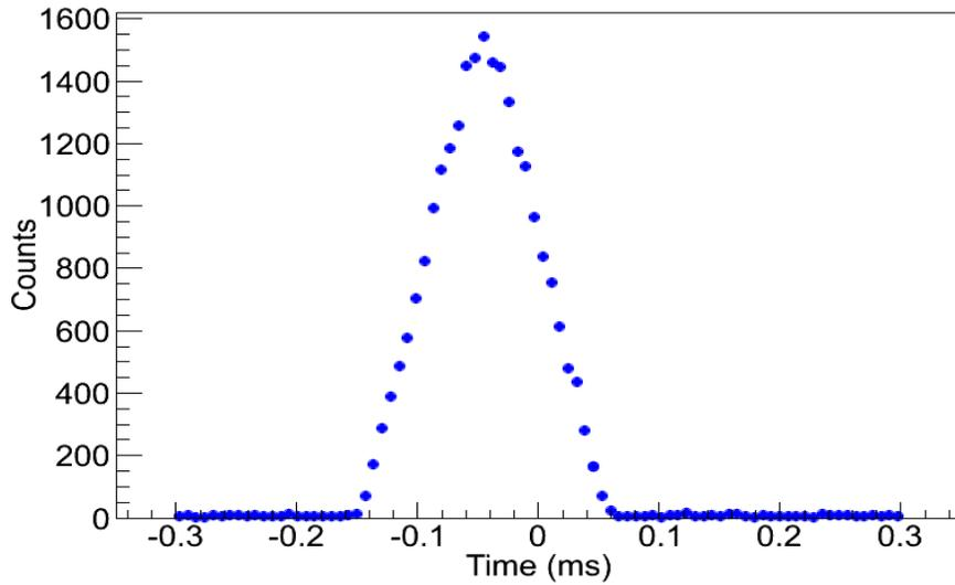
Fig. 4. Time coincidence spectrum between Timepix and the  $\Delta E$  detector
