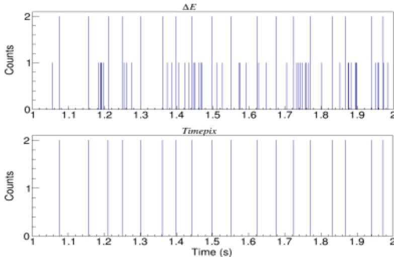
Fig. 2. Coincidence spectra when triggering Timepix from the  $\Delta E$  detector. A  $^{244}\text{Cm}$  alpha source was used.
