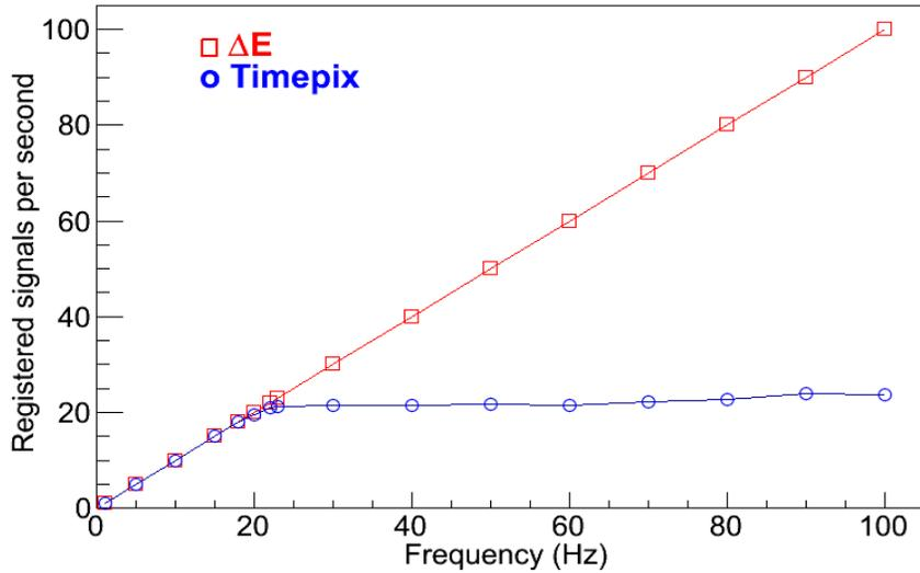
Fig.1. Dependence of registered signals on frequency. A test laser was used.
