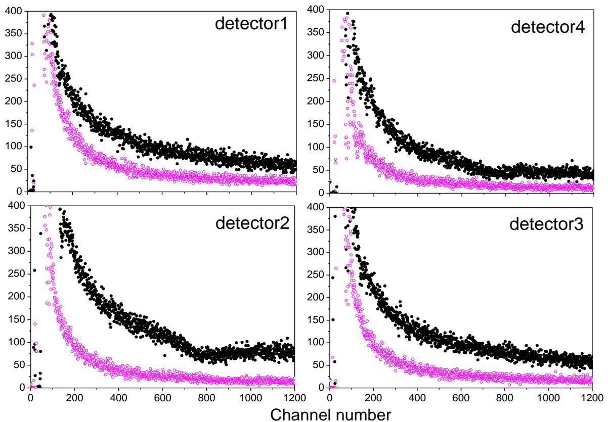
Fig.8. Time-of-flight spectra of neutrons obtained for neutron scattering by acrylic plastic at the scattering backward (open pink points) and forward (solid black points). Width of time channel is 0.5 mcs.
