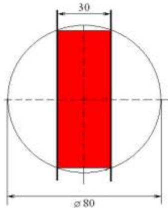
Fig.4. Placement of  $^3\text{He}$ -counter in the neutron beam. The beam direction is perpendicular to the figure flat.
