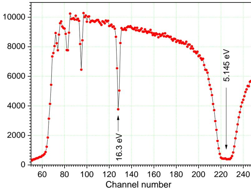
Fig.3. Segment of neutron spectra of monitor counter with resonance crevasses of silver 5.145 eV and 16.3 eV. Width of the time channel is 2 mcs.
