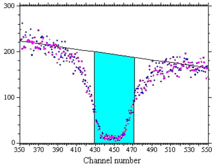
Fig.5. Neutron spectrum in the energy region 5 eV measured during 5 min. The blue area marks the interval between 428 and 471 channels, which corresponds to  $\Delta E=1$  eV. Width of the time channel is 1 mcs.
