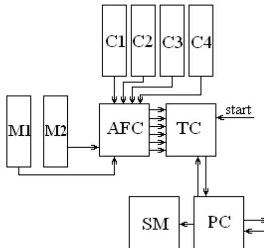
Fig.2. Scheme of the measuring module of the AURA setup. C1, C2, C3, C4 are detectors with preamplifiers, M1, M2 are monitor counters with preamplifiers, AFC is amplifier-former-signal converter unit, TC is time-coder, SM is stepper motor, PC is computer.
