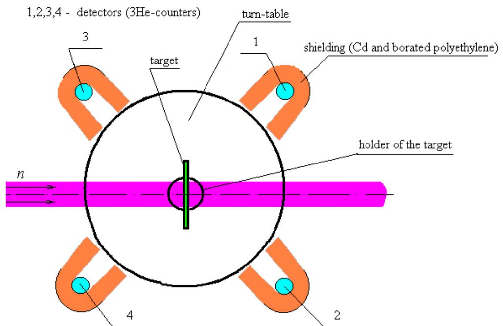
Fig.1. Scheme of the detecting module of AURA setup for the solid samples investigating.
