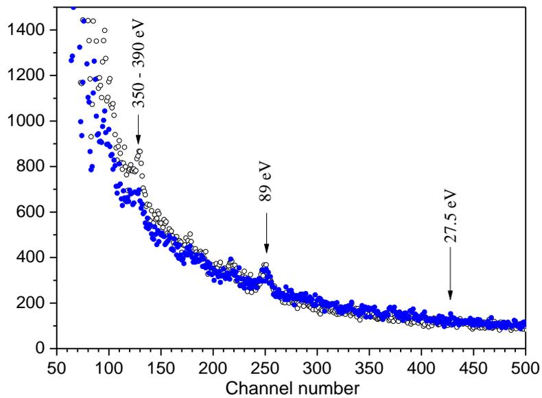
Fig.6. Time-of-flight spectra of neutrons scattered by Cd obtained with the 1-st detector at the neutron scattering backward (open points) and at the scattering forward (blue solid points). Width of the time channel is 0.5 mcs.
