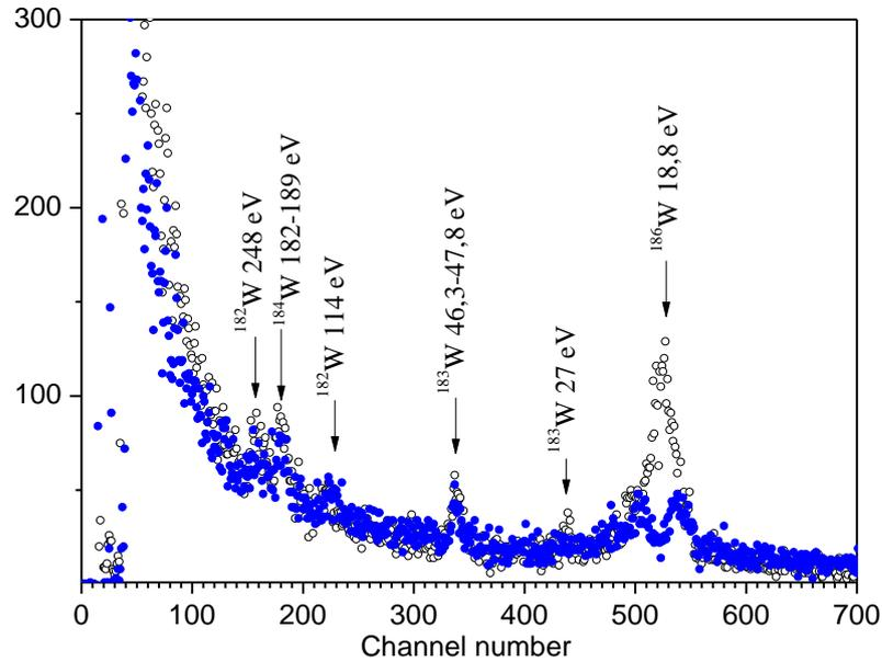
Fig.7. Time-of-flight spectra of neutrons scattered by W obtained with the 1-st detector at the neutron scattering backward (open points) and at the scattering forward (blue solid points). Width of the time channel is 0.5 mcs.
