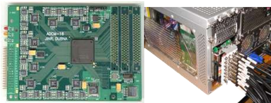
Fig. 2. The multichannel ADCM-16 board (left) and 2 boards in a computer, to form a 32 channel ADC system (right).
