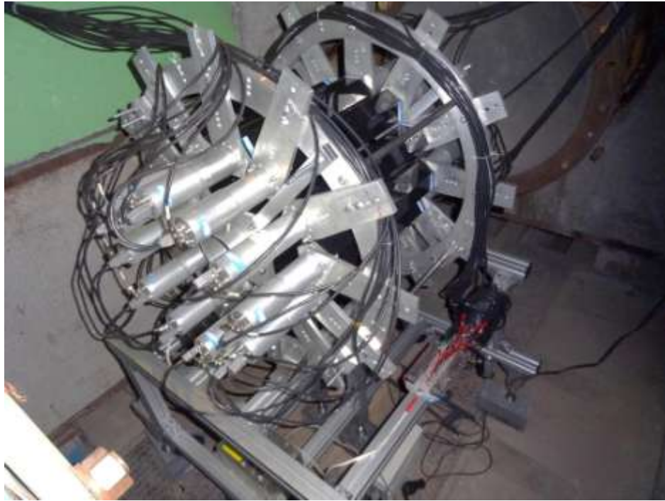
Fig. 1. Multi-detector gamma-ray spectrometry system: Two arrays of 12 NaI(Tl) detectors, Hamamatsu PMT+HV generator, HV generator power supply.
