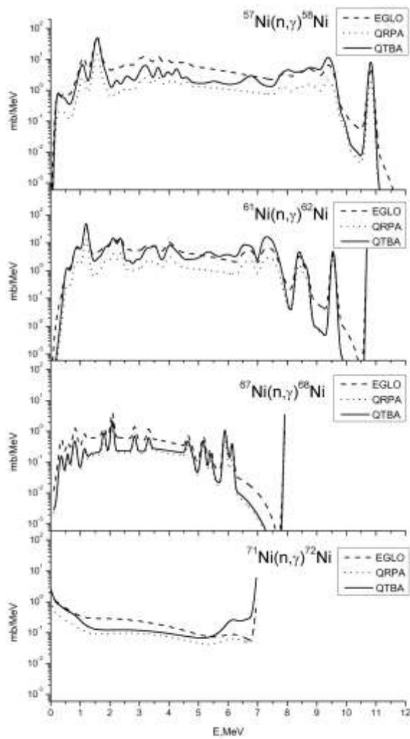
**Fig. 1.** Neutron capture gamma-ray spectra of Ni isotopes: microscopic QRPA (dots), and QTBA (solid line) and the phenomenological version EGLO (dashed). The incident neutron energy is 100 keV.
