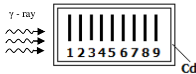
Fig.3. The arrangement of the samples. 1, 3, 5, 7 and 9 are the Cu; 2 and 4 are the Au; 6 and 8 are the Mo.
