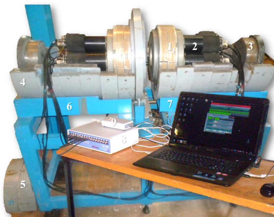
Fig. 1. Twelve crystal gamma-ray spectrometry system "Romashka": 1 – Six NaI(Tl) crystals in a single aluminum cylinder wrapped with aluminum arc-seals, 2 – Photo multiplier tubes FEU-110 and high-voltage divider, 3 – Lead shielding-collimator, 4 and 5 – Lower and upper lead shielding arcs, 6 – Adjustable rigid iron support, 7 – Movable iron trolley, 8 – 16 channels HVSys power supply [3], 9 – Parsek Desktop 8k MCA [4].
