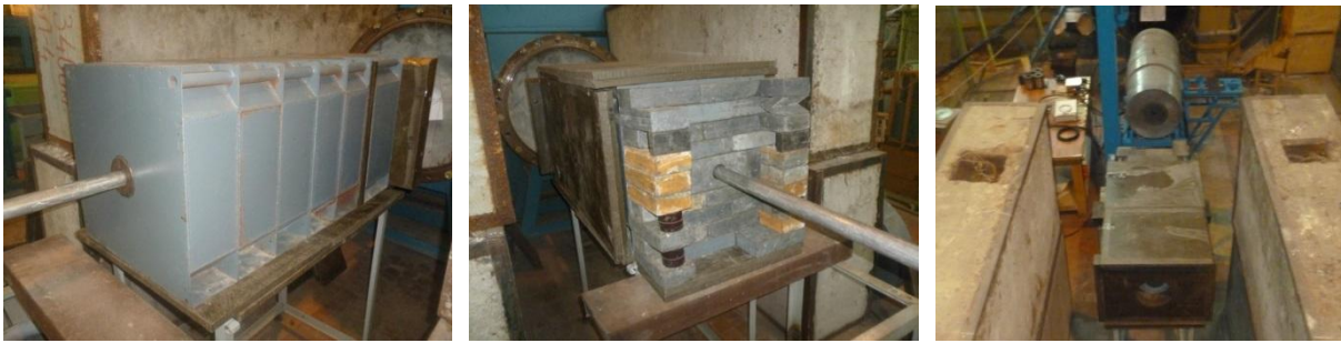
Fig. 2. Collimator canisters filled with different mixtures of materials (left), general view of the complete collimator from behind (middle) and general view of “Romashka” setup at the beam line (right).
