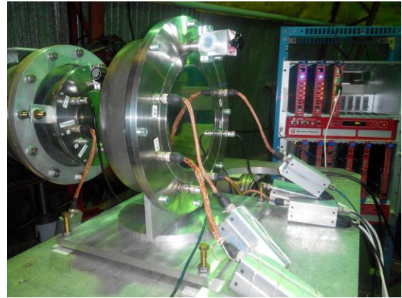
Fig. 4. View of the reaction chamber on the neutron beam.
