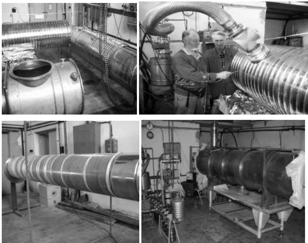
Fig. 2. Creation of an installation for measuring asymmetries of a neutron decay. (Superconducting solenoid, helium cryostat.)
