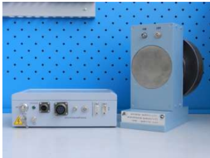
Fig. 3. ING-27 – neutron generator with built-in 192 pixel alpha-detector.
