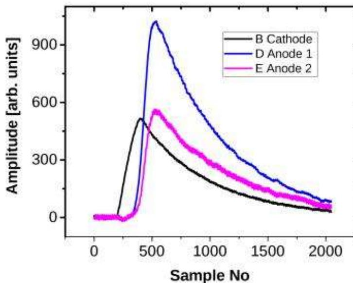
FIGURE 2. Original waveforms of the TIC cathode and anodes pulses.
