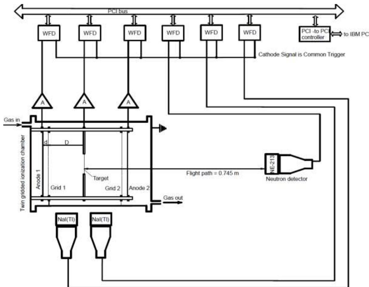
FIGURE 1. Sketch of experimental setup with digitizers.
