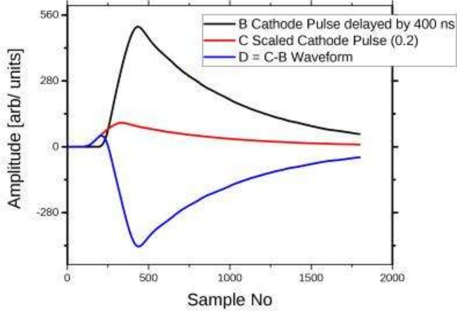
**FIGURE. 5.** Demonstration of the digital CFD realization. The zero crossing of the resulted bipolar signal was assigned the time mark.
