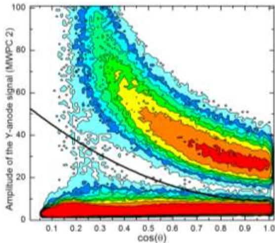
Fig. 3. Dependence of the amplitude of the Y-anode signal of MWPC 2 (D2) on the angle between fission fragment momentum and normal to the anode plane ( $^{233}\text{U}$ ). The “useful” events are located above the separation line (black).
