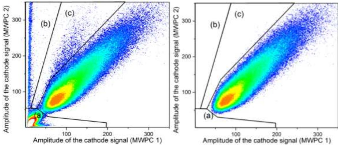
Fig. 5. A two-dimensional plot of the amplitudes of the cathode signals from two MWPCs in  $^{233}\text{U}$  experiment. The area of non-fission reaction products is labeled as (a). The fission events produced in the target are labeled: (b) - if fission fragments do not reach MWPC 1 (D1) due to limited transparency of MWPC 2 (D2); (c) - if the fragments do not pass through the cathode of the MWPC 1 (D1). Right part of this figure shows only “useful” data (for explanation see the text).
