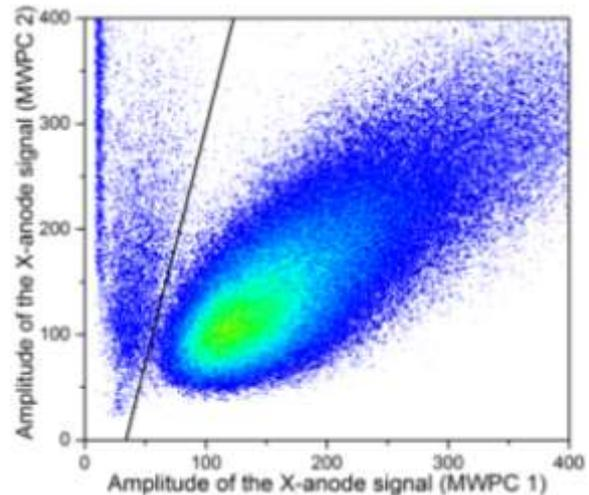
Fig. 4. Correlation between amplitudes of the X-anode signals of two MWPCs ( $^{233}\text{U}$ ). The “useful” events are located to the right of the separation line.
