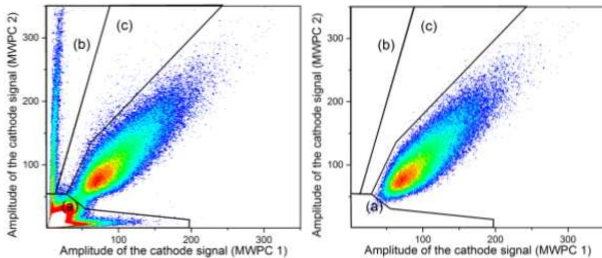
Fig. 6. A two-dimensional plot of the amplitudes of the cathode signals from two MWPCs in  $^{209}\text{Bi}$  experiment. Comments to this figure are the same as in Fig. 4.
