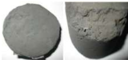
Figure 14. Air holes in materials.
