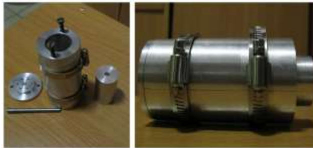
Figure 10. The mold for once-formation of compound materials.
