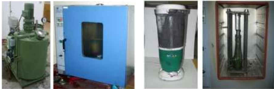
Figure 13. Instruments for experiments. From left to right: vacuum evacuation machine; incubator; mixer; screw jack and mold.
