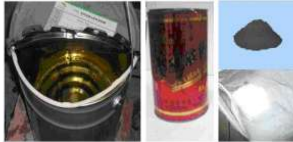
Figure 12. Materials for experiments. Left: bisphenol A resin E-51. Middle: polyamide 650. Right: tungsten and titanium dioxide.
