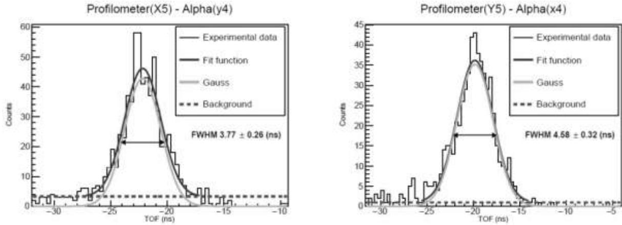
Fig. 8. Time spectra of the coincidences of signals between both X and y (left), and Y and x (right) strips of the neutron profile meter and alpha detector.
