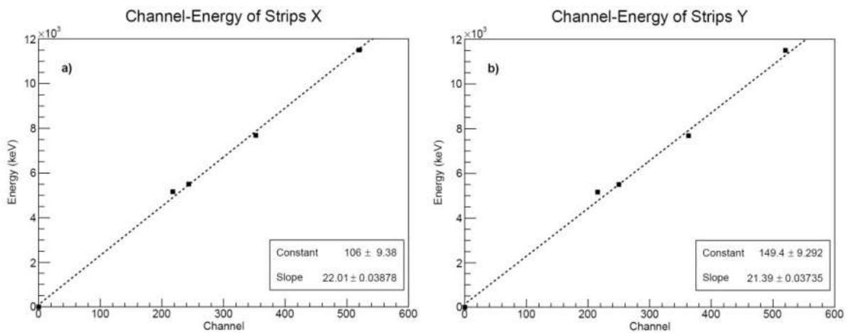
Fig. 5. Energy calibration of the profilometer X and Y strips, obtained with the following sources of alpha particles:  $^{239}\text{Pu}$  ( $E_\alpha = 5.2$  MeV),  $^{238}\text{Pu}$  ( $E_\alpha = 5.5$  MeV),  $^{226}\text{Ra}$  ( $E_\alpha = 7.8$  MeV) and  $^{28}\text{Si}(n, \alpha)^{25}\text{Mg}$  ( $E_\alpha = 11.5$  MeV).
