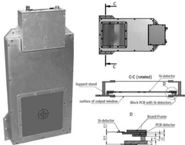
Fig. 4. Profilometer construction.
