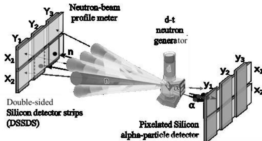
Fig. 7. The scheme of setup for measuring tagged neutron beam profiles.
