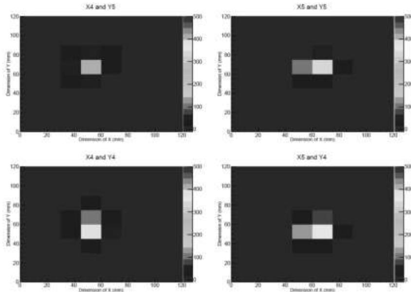
Fig. 9. Profile of the tagged neutron beam obtained at a distance of  $\sim 10$  cm from ING-27 neutron producing target.
