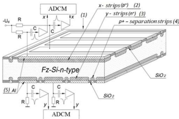
Fig. 3. The design of the integral double-sided silicon strip detector (DS-strip) and detector switching-on circuit with reading electronics.
