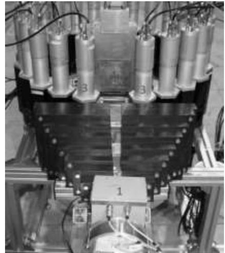
Fig. 1. Experimental setup: 1- the ING 27 neutron generator; 2 - the filter (passive shielding); 3 - the scintillation detector based on a NaI(Tl) crystal; 4 – the silicon two-dimensional position-sensitive fast neutron detector.
