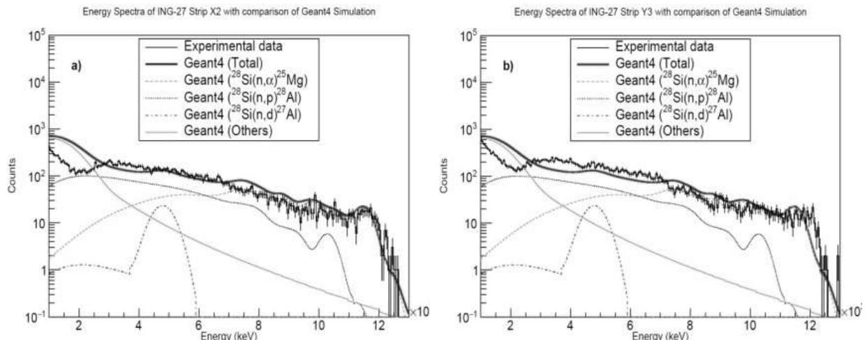
Fig. 6. Experimental and calculated energy spectra of the charged components obtained by irradiating X and Y strips with ING-27 tagged neutron flux. The calculated spectra are the result of simulation using Geant4 software.
