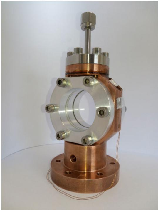
*Figure 3. Copper sample container with transparent amorphous silica ( $\text{SiO}_2$ ) windows used to obtain the UCN scattering cross sections presented in Section V.*
