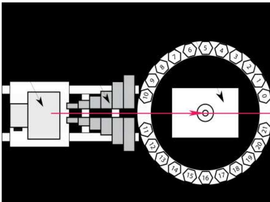
**Fig. 1.** Scheme of the TANGRA setup in the reaction plane: 1 – portable neutron generator ING-27, 2 – iron shielding, 3 – ”Romashka”  $\gamma$ -ray registration system, 4 – sample holder, 5 – setup frame. Arrow of the longitudinal line shows the neutron beam direction.
