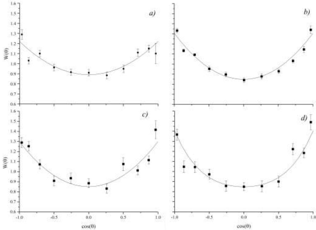
**Fig. 6.** The experimental angular distributions of  $\gamma$ -rays with energy  $E_\gamma = 1.014$  MeV (a),  $E_\gamma = 1.72$  MeV (b),  $E_\gamma = 2.21$  MeV (c) and  $E_\gamma = 3.004$  MeV (d) from inelastic scattering of 14.1 MeV neutrons by  $^{27}\text{Al}$ . Solid lines are approximations by Legendre polynomials.
