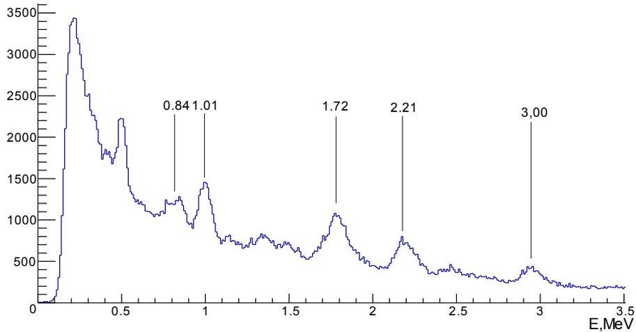
**Fig.5.** Gamma-ray energy spectrum emitted by  $^{27}\text{Al}$  during 14.1 MeV neutron irradiation.
