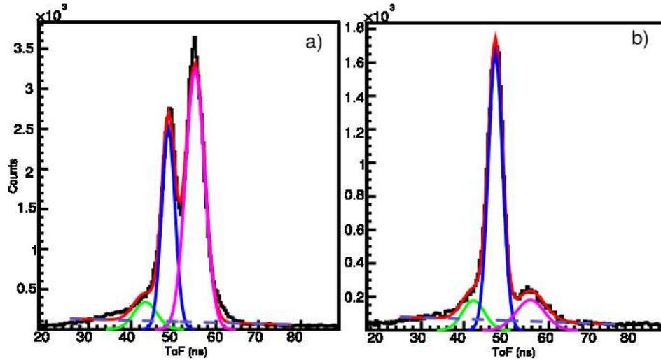
**Fig. 2.** Time-of-flight spectra and their approximations for  $\gamma$ -detectors placed at  $\sim 15^\circ$  (a) and  $\sim 90^\circ$  (b). The left peak corresponds to  $\gamma$ -quanta emitted from the neutron inelastic scattering in shielding, the central peak corresponds to the  $\gamma$ -quanta emitted from sample and the right peak is from the neutrons, which are elastically or inelastically scattered by the target.
