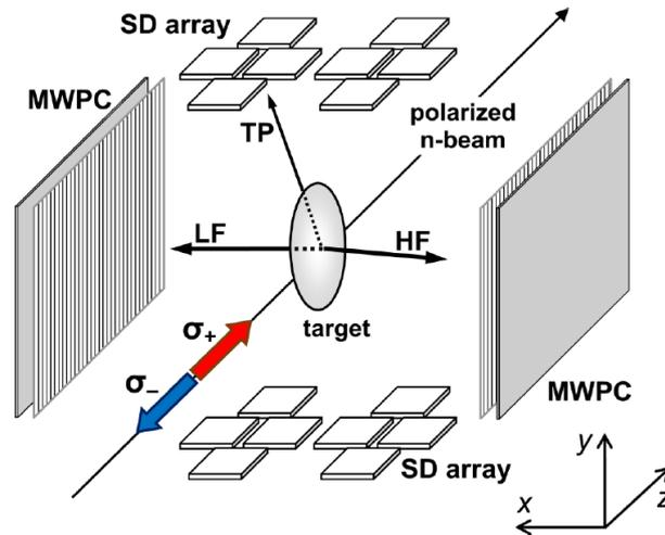
**Fig.3.** Layout of the experimental setup: fissile target locating at the center; polarized neutron beam running horizontally; two MWPC detecting complementary fission fragments to the left and right of the target, two arrays of Si detectors on top and bottom of the target intercepting ternary particles. All centers of particle detector assemblies lie in a plane perpendicular to the beam.
