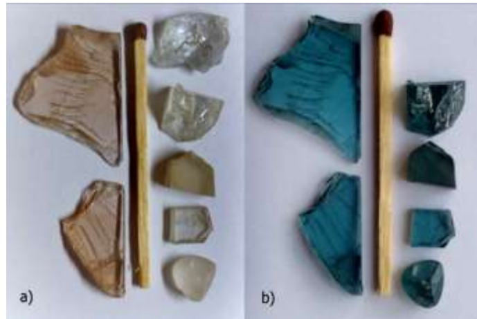
Fig. 1. Color changes of Ural topazes before (a) and after (b) neutron irradiation at the reactor IBR-2. Fast neutron fluence was about 10^{18} \text{ cm}^{-2} .
