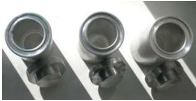
Fig. 5. The irradiation containers filled with boron carbide between aluminum layers
