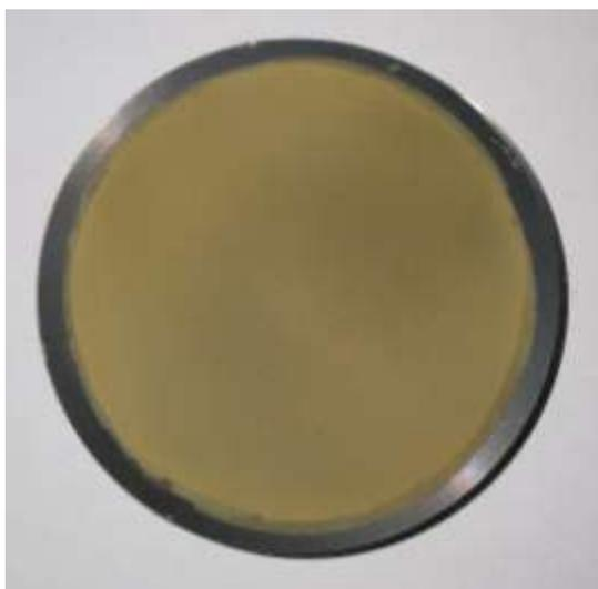
**Fig. 2** (Color online) Picture of the  $^{232}\text{Th}(\text{OH})_4$  sample.
