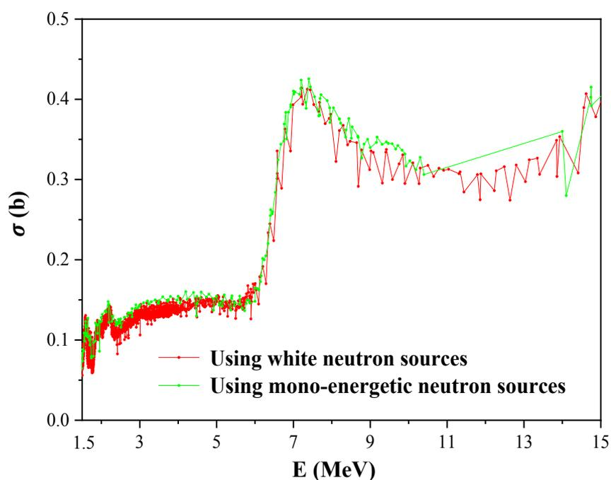
**Fig. 1** (Color online) Experimental cross sections of the  $^{232}\text{Th}(n, f)$  reaction from 1.5 to 15.0 MeV using white neutron sources and mono-energetic neutron sources. The results were taken from EXFOR library (after 1970s).
