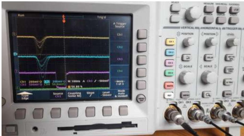
Fig. 14: testing of scintillator signals using Co-60 gamma ray source.
