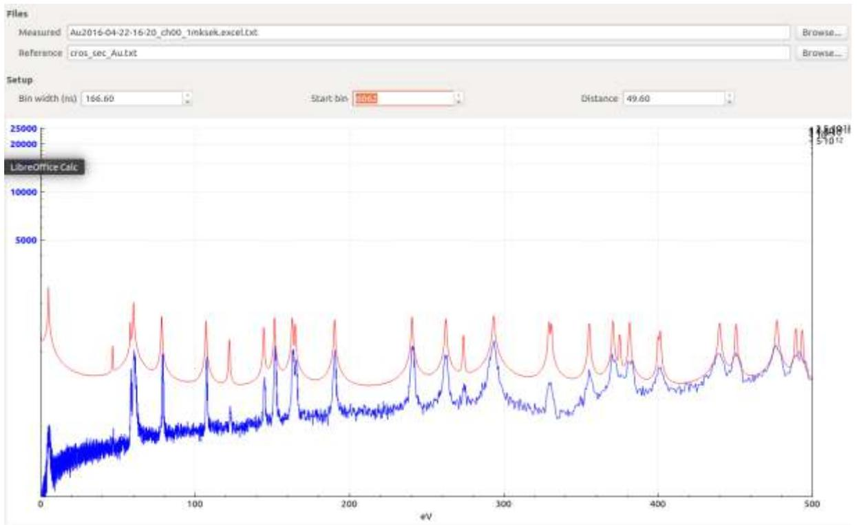
Fig. 11: Au-197 cross capture, beam pulse duration 1 mks.
