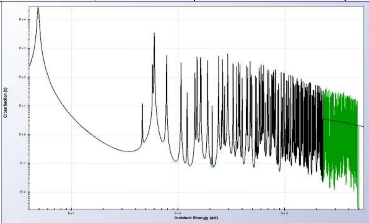
Fig. 10. Capture cross section of Au-197.
