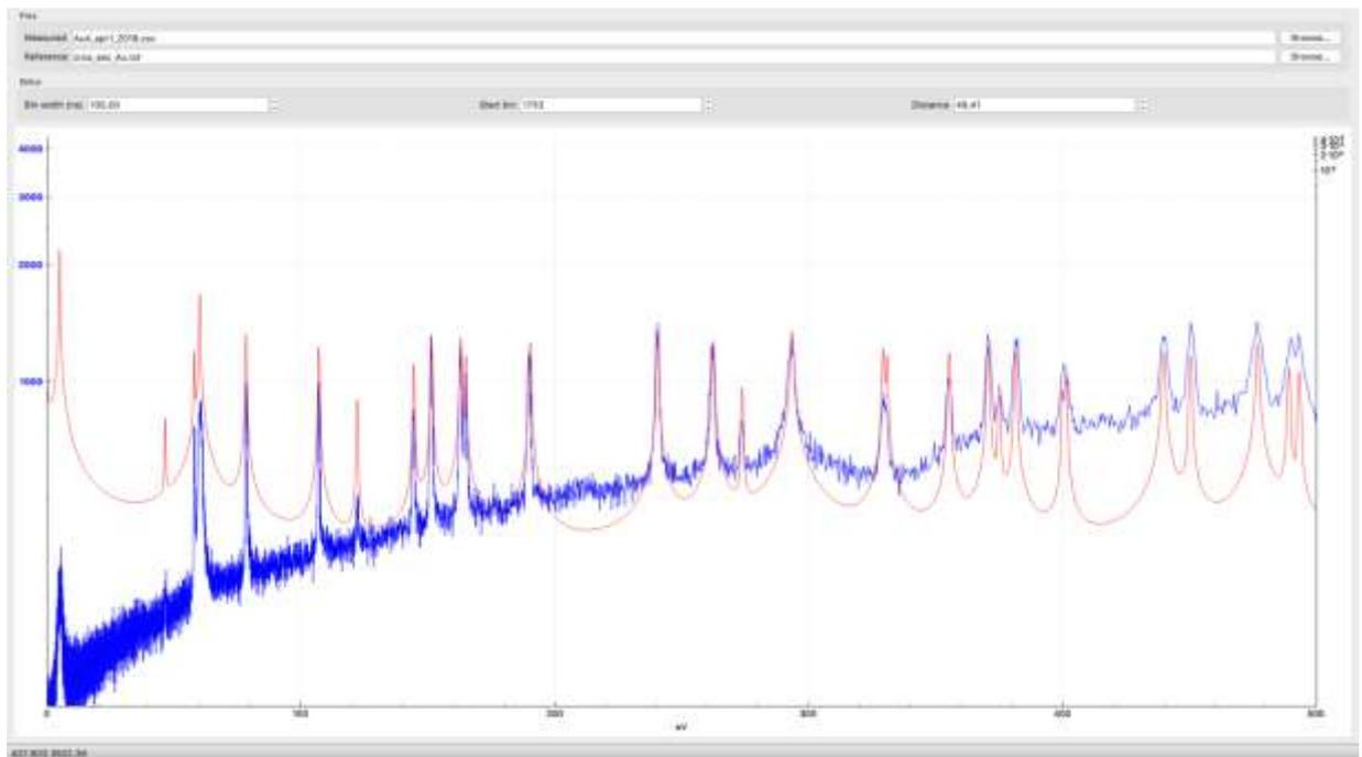
Fig. 12: Au-197 capture cross section, beam pulse duration 500 nanoseconds.
