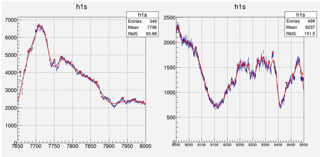
Fig. 9: Ta-181 unresolved capture resonance area after the proton beam flash.
