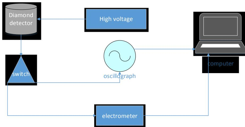
Fig. 3. Diamond detector measuring circuit.
