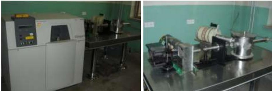
**Fig.4** Philips X'Unique II X-ray source. It is a bremsstrahlung X-ray spectrometer with maximum voltage 100 kV, maximum current 60mA and rated power 3 kW. X-rays are generated by accelerated electrons stopped by W target. The right picture is HPGe detector used in experiments.
