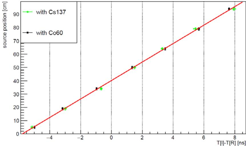
Fig. 8. Measured time difference versus the position of the radiation source for the EPIC detector. Experimental data were obtained with a  $^{60}\text{Co}$  source (squares) and with a  $^{137}\text{Cs}$  source (circles). The solid line is the fit of a linear function to the experimental data.
