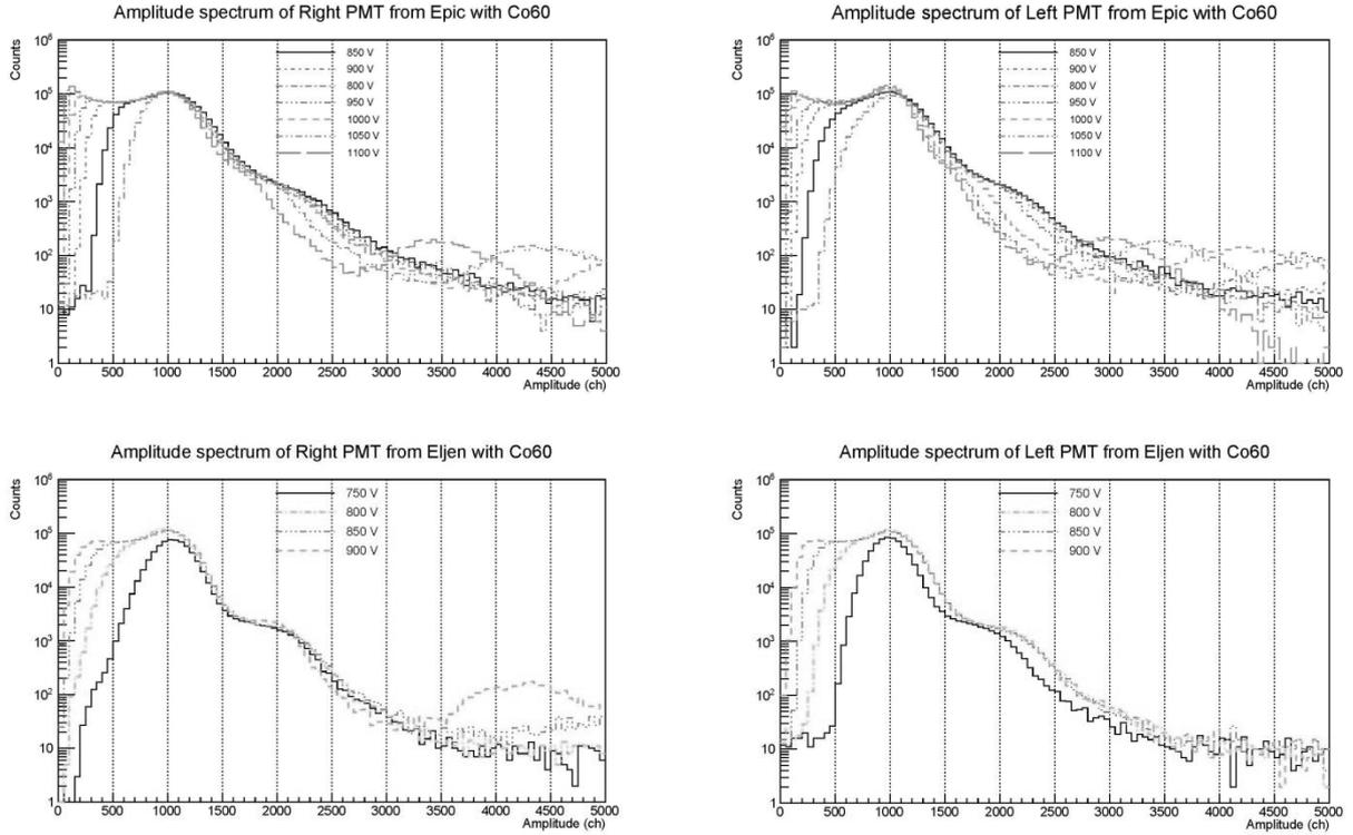
Fig. 3. Amplitude spectra of the right and left photomultipliers from the EPIC CRYSTAL and ELJEN TECHNOLOGY detectors.
