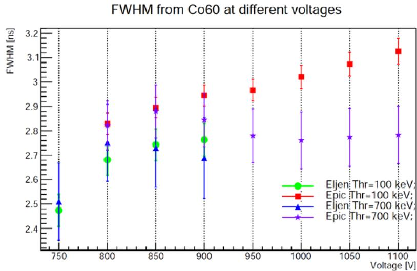
Fig. 6. FWHM of the time peak versus PMT voltage for the EPIC and ELJEN detectors with thresholds 100 and 700 keV.
