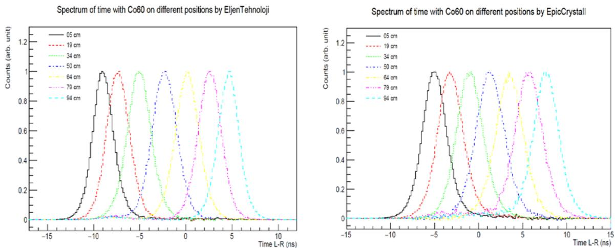
Fig. 7. The time difference spectra, obtained with  $^{60}\text{Co}$  radioactive sources and collimator assembly for various distances of the exposed part from one end by the ELJEN (left) and EPIC (right) detectors.
