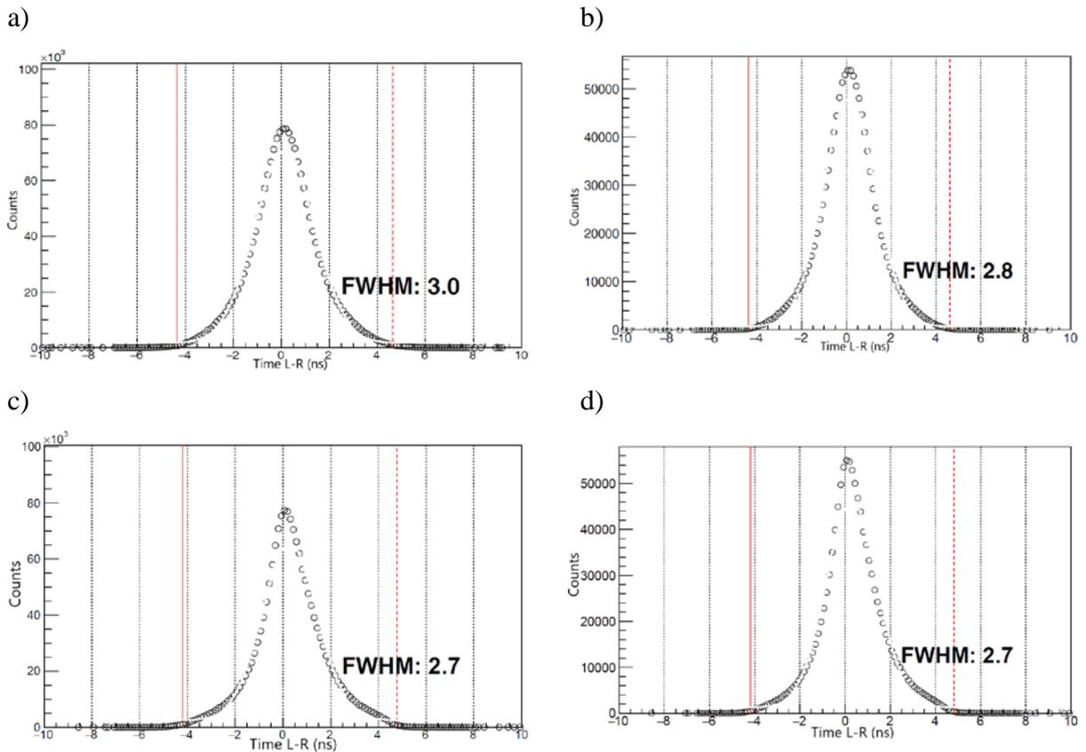
Fig. 5. Time spectra ( $T_L-T_R$ ) for detectors: EPIC at a voltage of 950 V and an interaction threshold  $E_{thr} = 100$  keV (a),  $E_{thr} = 700$  keV (b) and ELJEN at a voltage of 850 V and an interaction threshold  $E_{thr} = 100$  keV (c),  $E_{thr} = 700$  keV (d).
