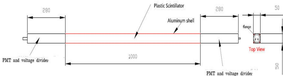
Fig. 2. The schematic view of the studied detectors [6].
