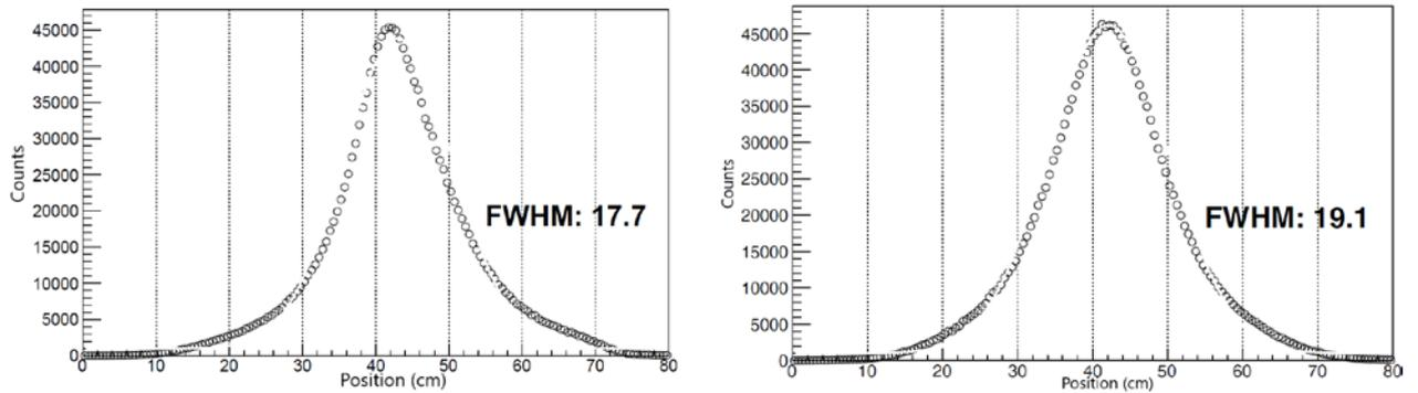
Fig. 9. Position resolution for ELJEN (left) and EPIC (right) detectors measured with a  $\gamma$  ray beam from a  $^{60}\text{Co}$  point source collimated using appropriately placed lead bricks to illuminate a 0.5 cm wide portion of the plastic scintillator.
