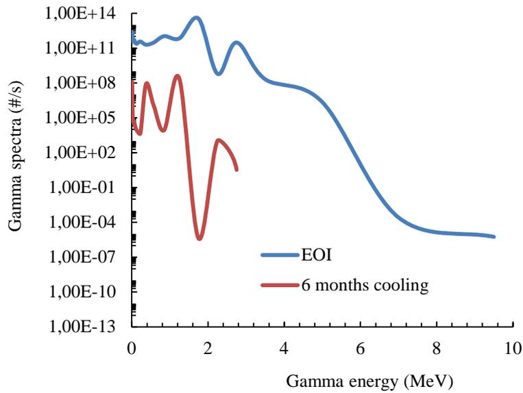
Figure 6: Comparison of Gamma spectra of the radioactive irradiation box at 6 months cooling time and EOI.
