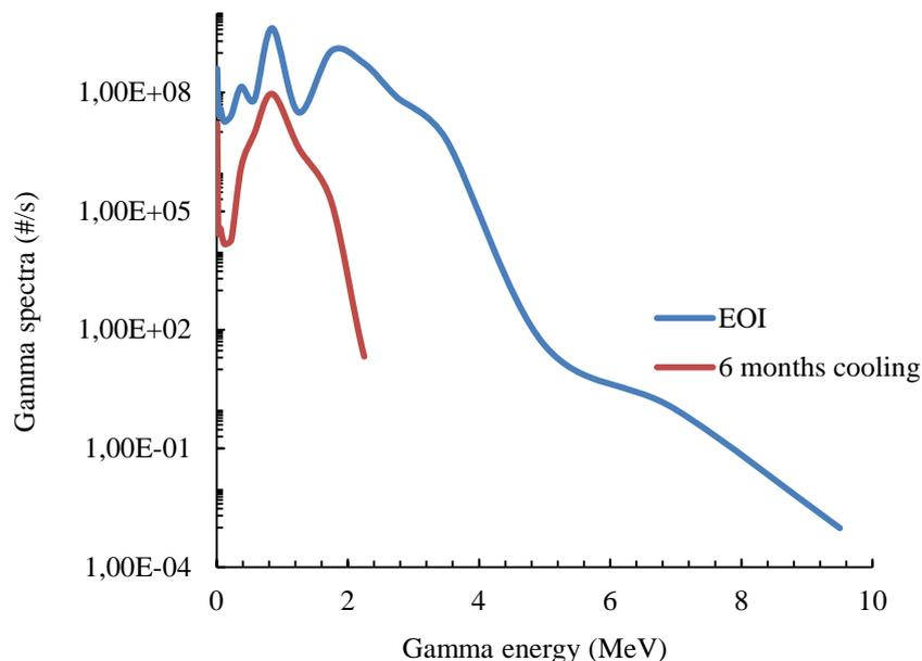
Figure 8: Comparison of Gamma spectra of the radioactive steel lining piece at 6 months cooling time and EOI.
