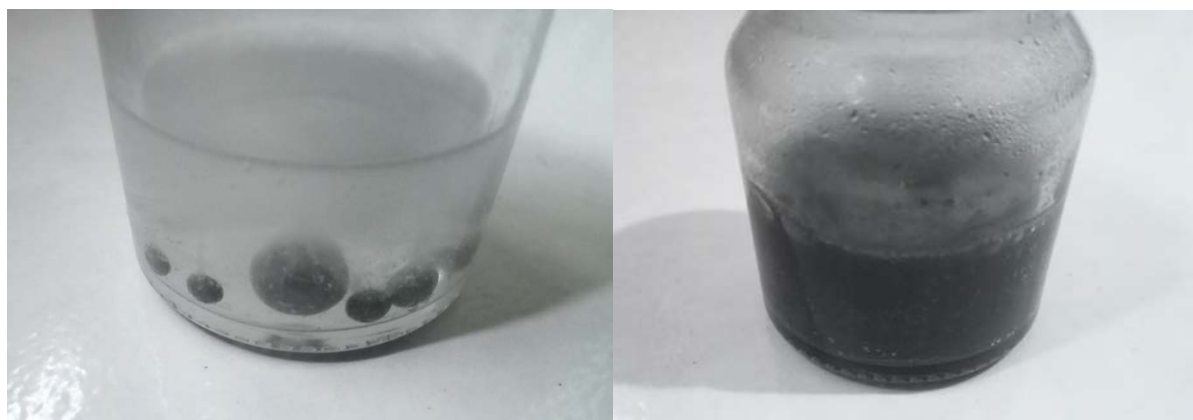
Figure 3: Dissolution of beryllium metal in peroxyacetic acid (left) and precipitation of bismuth beryllium acetate (right).
