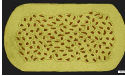
Figure 2. LEU fuel rod cross section.
