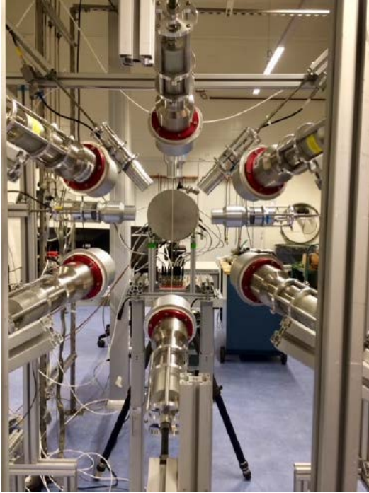
Fig.1. The experimental setup from behind the neutron detector array.
